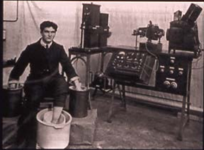
The first complete Cambridge electrocardiograph apparatus in 1911. From right to left, arc lamp, string galvanometer and two cameras. The camera on the left has an oil-damped falling plate, and the one on the right is a continuous paper camera.
