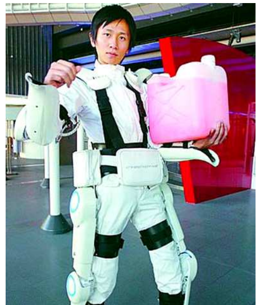
Figure 14 HAL-5 lifting a 40kg gallon ( http://obychnogo.net )
