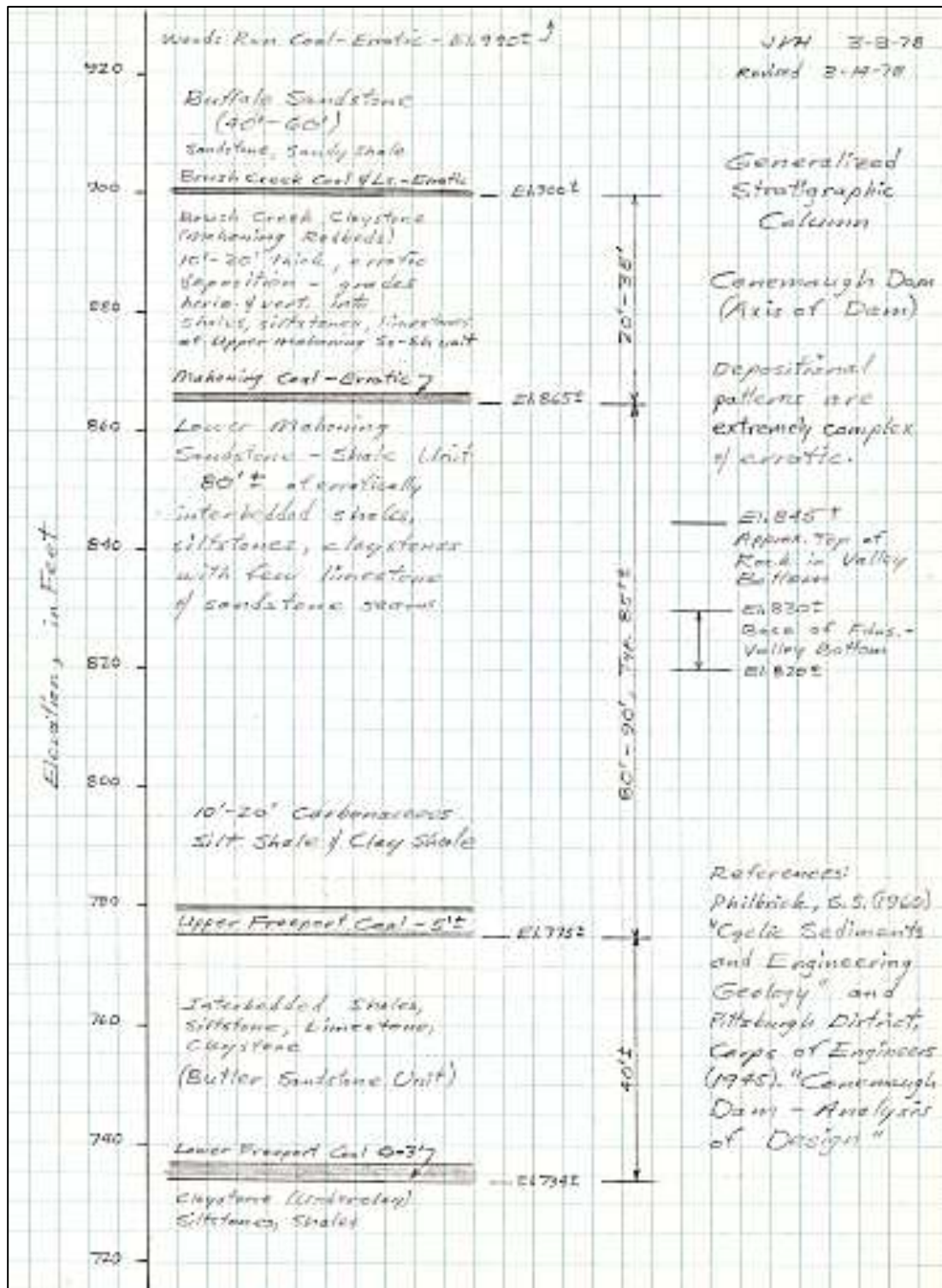
Stratigraphy of the lower Glenshaw Formation deposits below Conemaugh Dam and Bow Ridge (1978) provided courtesy of James Hamel. The stratigraphic interpretation shown here was based on work done in the 1930's and 1940's by Shailer Philbrick, one of the founders of the Pittsburgh Geological Society.
