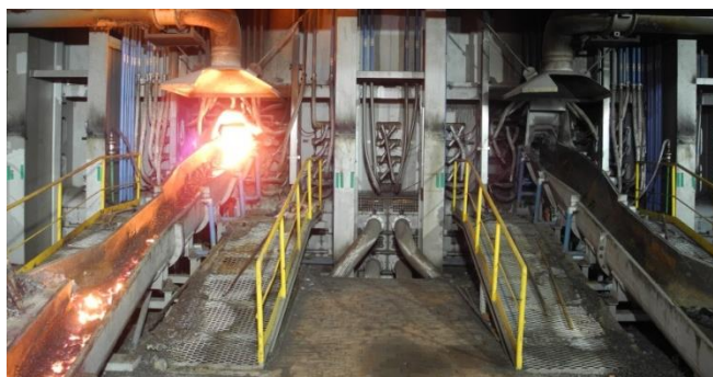
Figure 3: Slag tapping at POSCO SNNC FeNi-furnace
