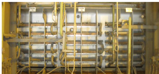
Fig. 1: Sidewall cooling concepts based on stripe cooling
