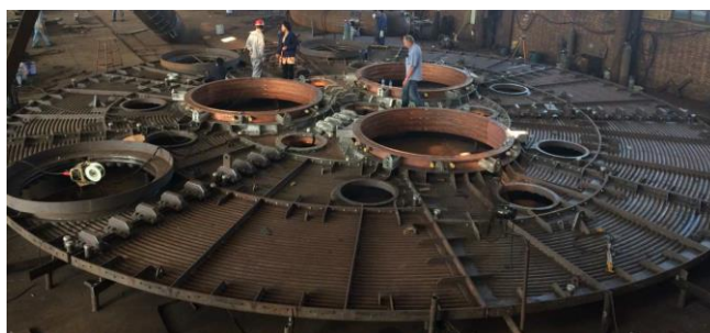
Figure 8: Water cooled roof during manufacturing for Rainbow Minerals
