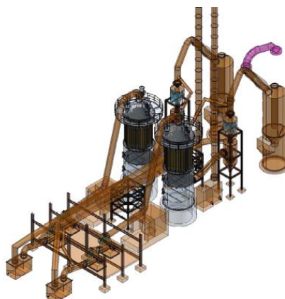
Figure 9: Wet gas cleaning plant for closed submerged arc furnaces
