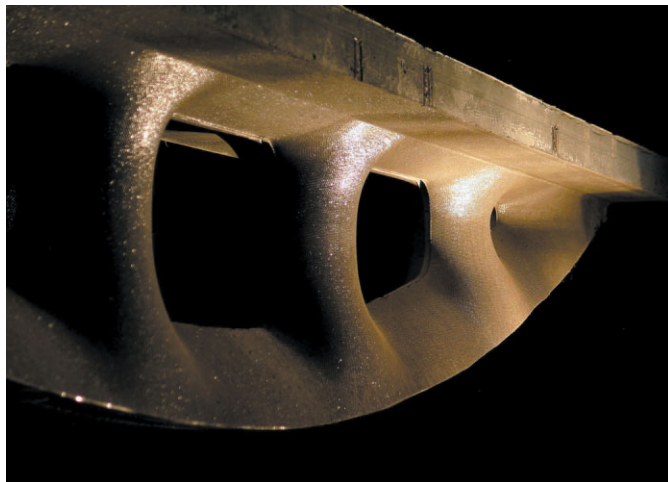
Fig. 21. Fabric-formed truss fabricated at C.-A.-S.-T.
