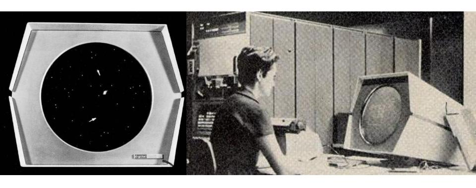
1963: For his doctoral thesis at MIT, Ivan Sutherland develops Sketchpad, the first Computer-Aided Drafting and Design (CADD) package allowing shapes to be interactively drawn on a vector-based display monitor using a light pen input device wired into the computer. The light pen uses a small photoelectric cell in its tip to emit an electronic pulse when the pen "sees" the electron beam.
