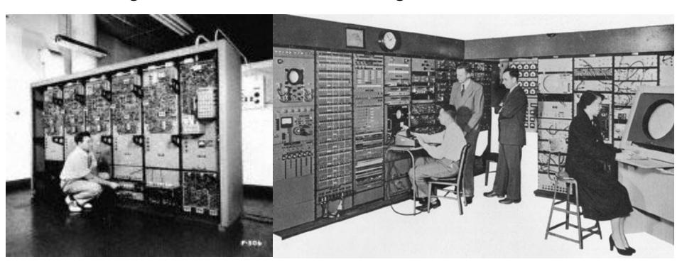
• 1955: Direct descendant of the Whirlwind, the SAGE (Semi-Automatic Ground Equipment) air defense system is designed by Bert Sutherland at MIT. It uses simple vector graphics to display on analog CRTs radar images with a wireframe outline of the region being scanned, as well as the first light pen as an input device that operators would use to pinpoint planes flying over regions of the United States. It becomes a key part of the US missile defense system.
