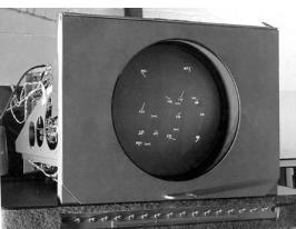
1959: General Motors and IBM develop "DAC-1" (Design Augmented by Computers), the first industrial CAD system (Computer-Aided Design) used to help engineers design cars. It allows a user to rotate and view a simple drawings.
