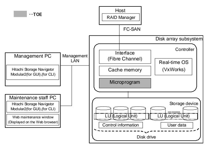
Figure 2 TOE Logical Configuration
