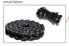
Since the machine had been engaged in heavy duty work for few days, few of the track links has cracked. They were replaced as individual parts as oppose to the track link assemble replacement.
