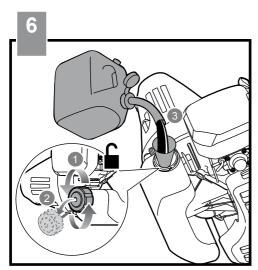
Loosen the fuel cap. Remove the fuel cap. Carefully pour fuel mixture into the tank. Avoid spillage. Immediately replace fuel cap and hand tighten.
