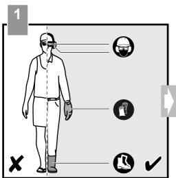
Always wear safety goggles or safety glasses with side shields when operating the product. Failure to do so could result in objects being thrown into your eyes resulting in possible serious injury. When handling the trimmer assembly, wear non-slip, heavy-duty protective gloves. Wear nonskid, protective footwear that will protect your feet and improve your footing on slippery surfaces.
