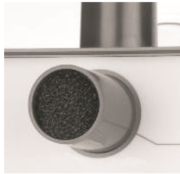
Figure 3-4: Filter at inlet of system
