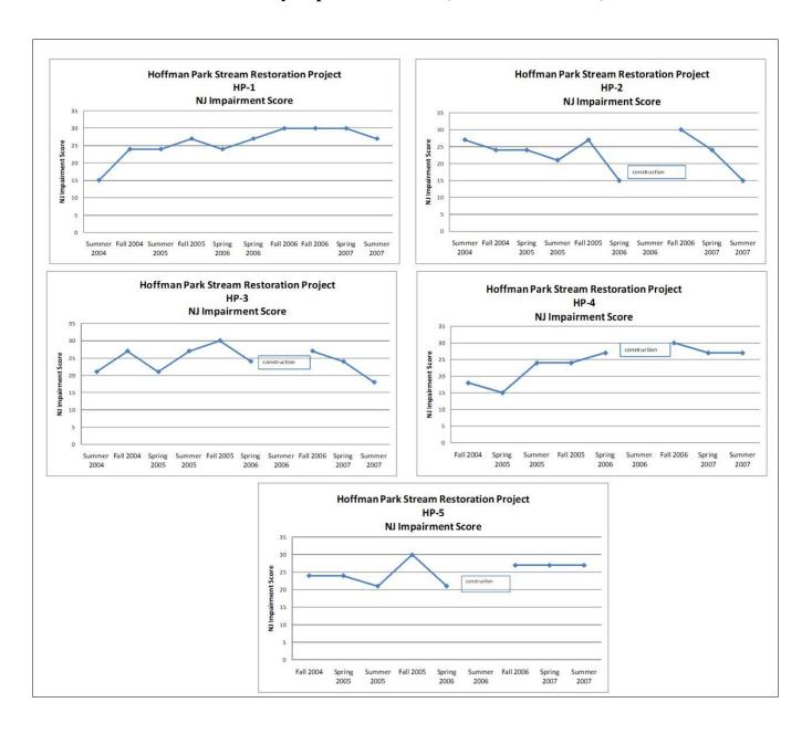
The habitat assessment indicated an improvement in the scores following the implementation of the restoration project. No assessments were conducted during Summer 2006 due to construction; therefore there is a break in the data reflecting construction.
