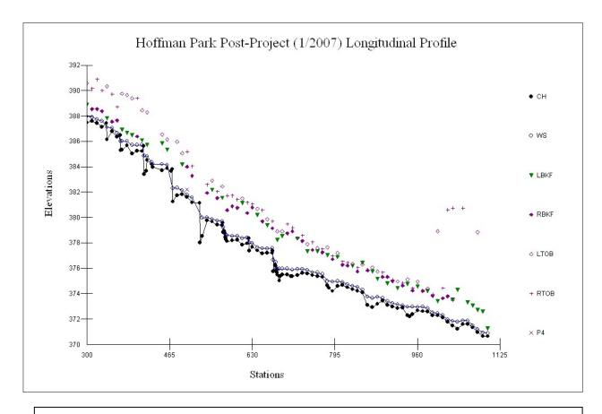
$CH-thalweg \quad WS-water\ surface\ elevation\ \ LBKF/RBKF-left/right\ bankfull\ depth\ \ LTOB/RTOB-left/right\ top\ of\ bank\ \ P1-P4-Other\ features$
