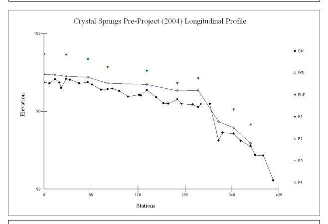
$CH-thalweg \quad WS-water\ surface\ elevation\ \ LBKF/RBKF-left/right\ bankfull\ depth\ \ LTOB/RTOB-left/right\ top\ of\ bank\ \ P1-P4-Other\ features$
