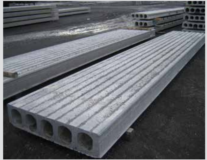
Longitudinally raked slab
