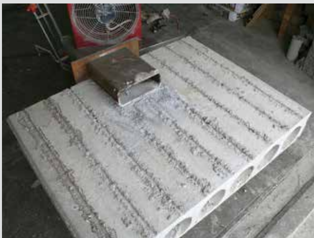
Structural steel assembly insert in dry-mix longitudinally raked specimen DRY-LRX-1
