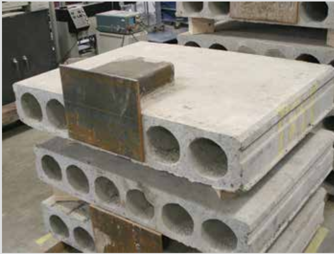
Specimen with machine-finished surface
