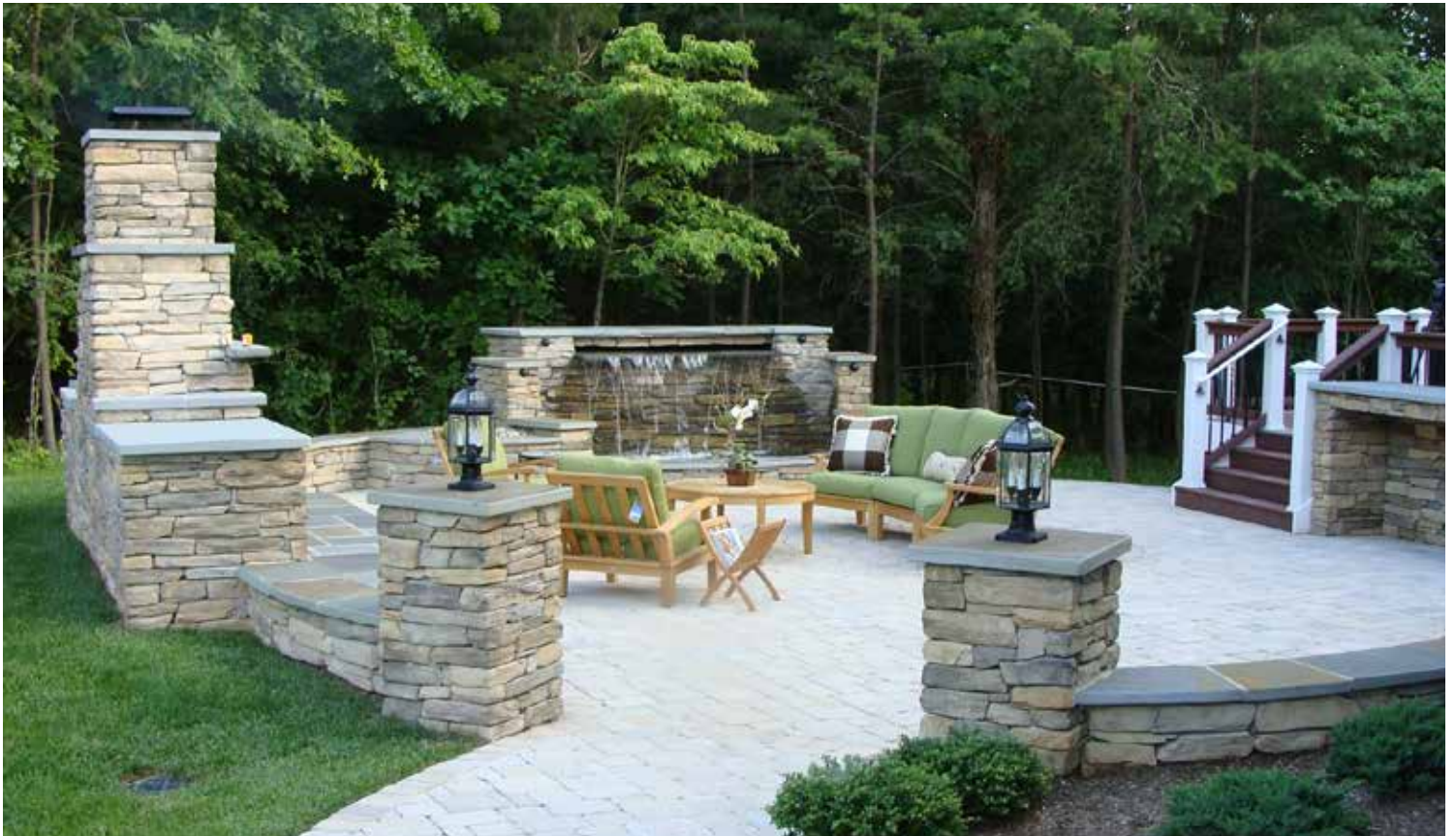
ABOVE: CULTURED VENEER DRY STACK WALLS AND COLUMNS WITH LIGHTS. 42" FIREBOX FIREPLACE WITH FIREBRICK INTERIOR. CUSTOM WATERFALL. HANOVER PATIO: CHISELED FINISH WITH TUMBLED FINISH DUAL EDGE PATIO. TREX TRANSCENDS DECK.
