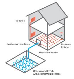
Layout of a typical geothermal heating system
