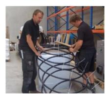
Manufacturing a 'slinky' ground loop pipe
