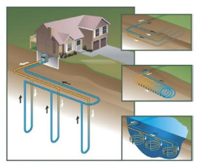
types of geothermal loops (clockwise from left) Vertical Loops, Horizontal loops, slinky loops and open loops.
