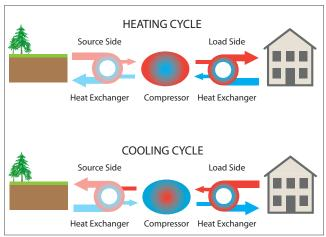
The three loops of the heating & cooling cycle
