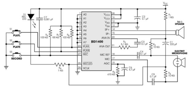
Note: We built a similar circuit from the above reference circuit with some modifications. First the Address bit A0-A7 will connect to our Mega32 PORTB. We also do not have pushbutton switches and unnecessaries LEDs.
