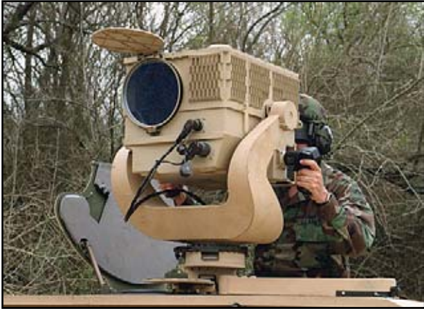
Fig. 3. The Long Range Advanced Scout Surveillance System (LRAS3) as mounted on a HMMWV's roof.
