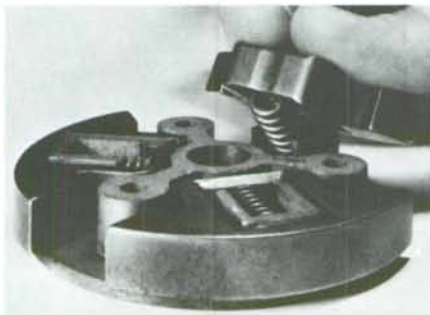
Fig. HL47—View showing easy method for installing late type clutch shoes and springs on clutch plate.
