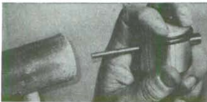
Fig. HL40—After removing snap rings the piston pin can be tapped out using a \frac{3}{16} inch (4.76 mm) rod as shown or, on pistons with Spirol pin at exhaust side, by driving piston pin out with slotted driver (Homelite tool A23949).
