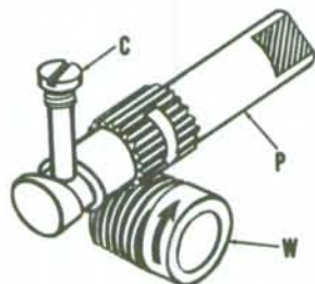
Fig. HL44—Automatic oil pump worm gear (W) driven by crankshaft turns plunger (P) at 1/20 engine speed. As plunger turns, cam on end of plunger engages cam screw (C) causing the plunger to go back and forth. Flat end of plunger acts as inlet and outlet valve.
