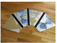
4. Tape the four pieces of cardboard together with duct tape or another heavy, durable tape. Then connect the far ends to complete the reflector.
