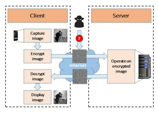
FIGURE 5.1: System Architecture of CryptoImg.
