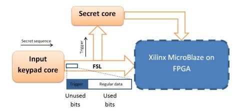
FIGURE 3.5: Block diagram of using a malicious secret core within an untrusted e-voting machine.
