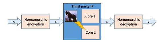
FIGURE 4.1: Homomorphic encryption to protect from Hardware Trojans.
