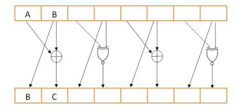
FIGURE 3.6: Simple obfuscating function depending on data xoring.
