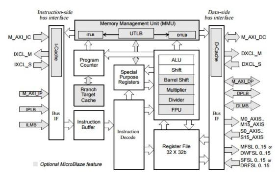
FIGURE 3.4: MicroBlaze block diagram [45].
