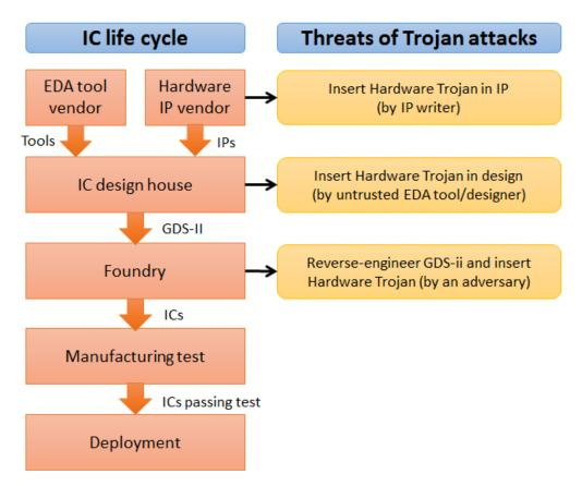
FIGURE 2.1: Possible stages for launching Hardware Trojan (HT) attacks by third parties during IC life cycle [25].
