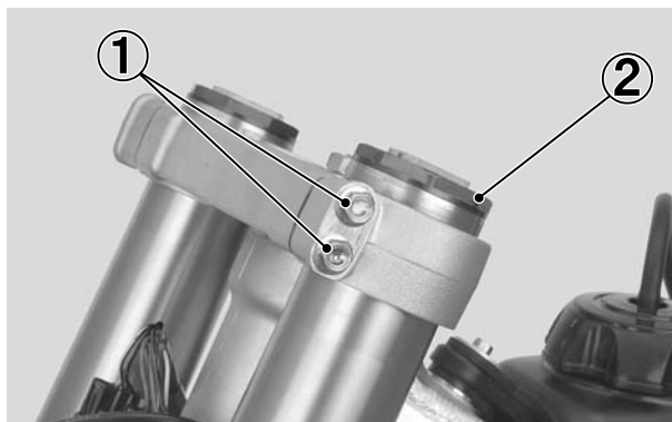
(1) UPPER PINCH BOLTS (2) FORK DAMPER
