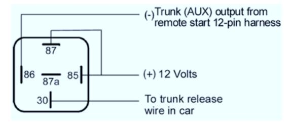
**NOTE:** the 12V source can be taken from the red wire on the 12 pin harness. Pin 87a on the relay is not used. Cut and cap that wire.
