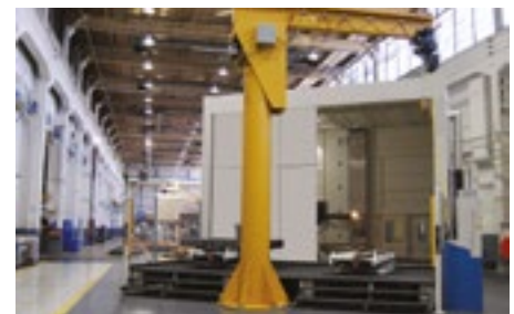
Full Enclosure with Roof and Mist Collector
