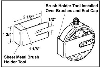
Figure 8-36. Brush Holder Tool (Style "A" End Cap).
