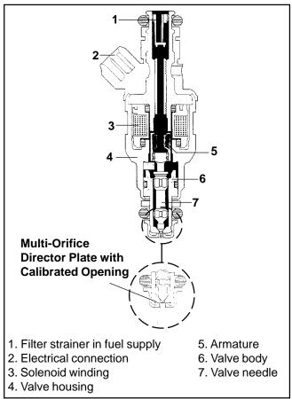
Figure 5B-18. Fuel Injector Details.
