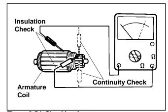
Figure 8-54. Checking Armature.
