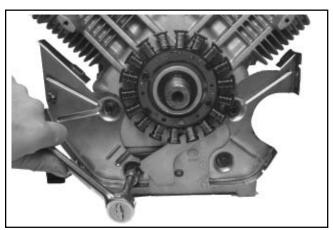
Figure 9-59. Removing Backing Plates and Stator Wire Bracket.
