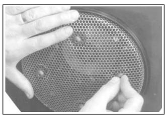
Figure 11-66. Installing Metal Type Grass Screen.
