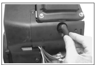
Figure 11-98. Connect Spark Plug Leads.
