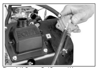
Figure 9-16. Remove Fuel Pump and Lines.
