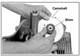
Figure 9-64. Removing Camshaft (Note Shim).
