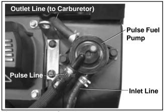
Figure 5-1. Pulse Style Fuel Pump.
