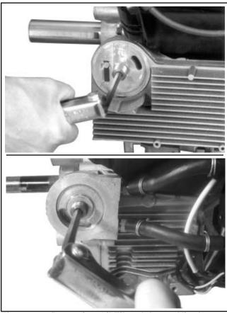
Figure 9-6. Removing Oil Filter Adapter Nipple.
