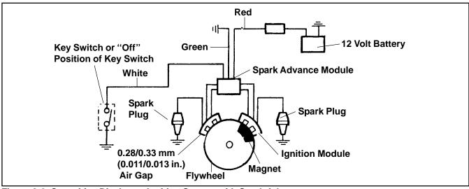
Figure 8-6. Capacitive Discharge Ignition System with Spark Advance.
