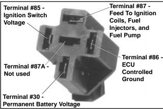
Figure 5B-14. Relay Connector.
