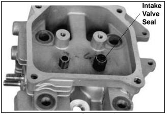
Figure 11-37. Intake Valve Seal Location.
