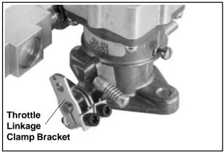
Figure 5A-13. Throttle Linkage Clamp Bracket Position.
