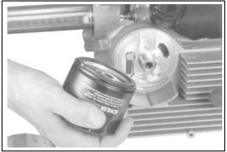
Figure 11-93. Installing New Oil Filter.
