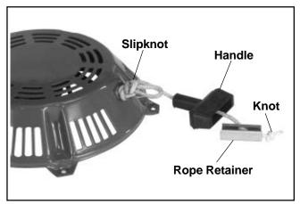
Figure 7-2. Removing Starter Handle.
