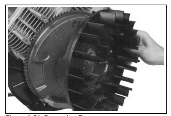
Figure 9-56. Removing Fan.
