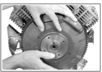
Figure 11-28. Carefully Align Keyway to Key.
