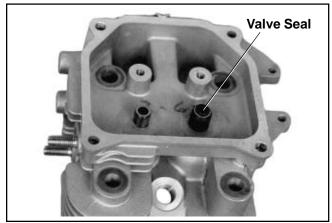
Figure 9-54. Intake Valve Seal Location.
