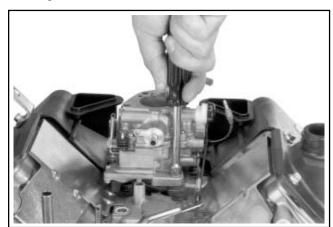
Figure 9-23. Removing Carburetor Mounting Screws.
