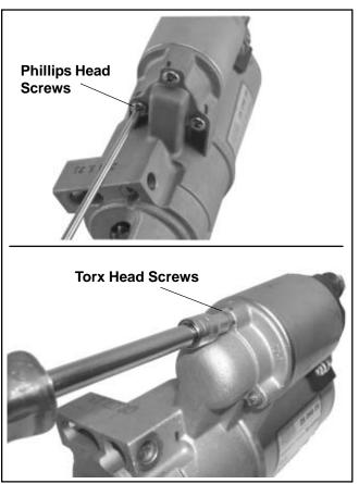
Figure 8-41. Removing Solenoid Screws.
