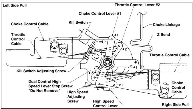
Figure 5-11. Governor Control Connections.
