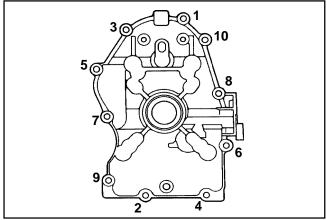
Figure 11-21. Closure Plate Fastener Torque Sequence.
