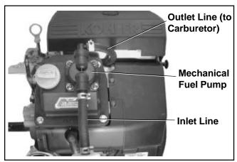
Figure 5-2. Mechanical Fuel Pump.
