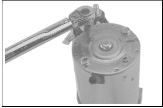
Figure 8-68. Torquing Brush Holder Screws.
