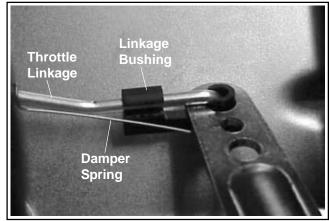
Figure 5B-37. Throttle Linkage/Governor Lever Connection.
