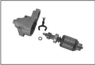
Figure 8-48. Armature and Lever Removed.
