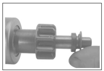
Figure 8-58. Installing Thrust Washer.
