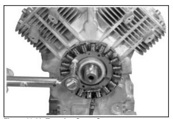
Figure 11-23. Torquing Stator Screws.
