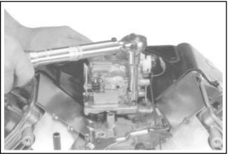
Figure 11-75. Installing Carburetor Assembly.
