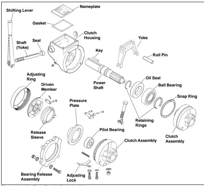
Figure 12-1. Wet Type Clutch - Exploded View.
