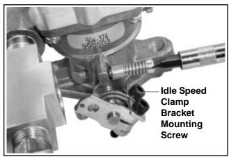
Figure 5A-8. Backing Off Idle Speed Screw.
