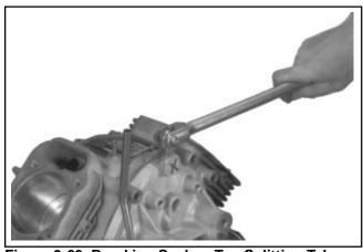
Figure 9-63. Breaking Seal on Top Splitting Tab.
