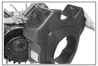
Figure 9-33. Removing Blower Housing.
