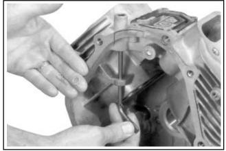
Figure 11-3. Installing 6 mm Governor Cross Shaft.
