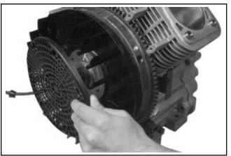
Figure 9-55. Removing Plastic Type Grass Screen.
