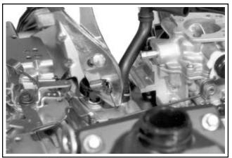
Figure 9-11. Removing Tube from Breather Cover.
