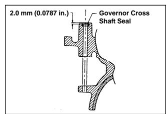
Figure 10-18. Installing Cross Shaft Oil Seal.
