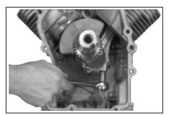
Figure 9-65. Removing Connecting Rod Bolts.
