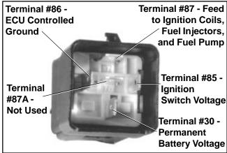
Figure 5B-15. Relay Terminal Details.
