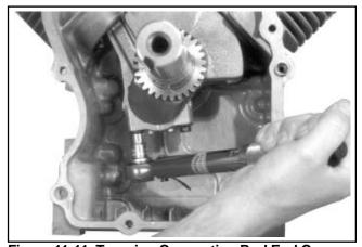
Figure 11-11. Torquing Connecting Rod End Cap.
