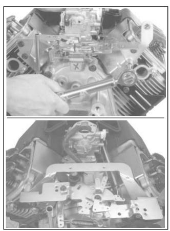
Figure 11-81. Torquing Main Control Bracket.
