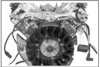
Figure 11-55. Connect Leads on SMART-SPARK<sub>™</sub> Ignition Modules.
