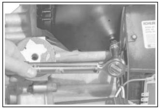
Figure 11-64. Tighten Short Screws to Torque Specified.
