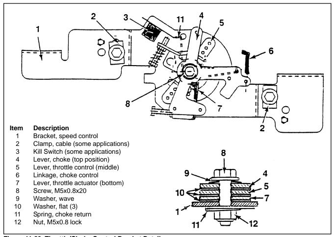
Figure 11-83. Throttle/Choke Control Bracket Detail.
