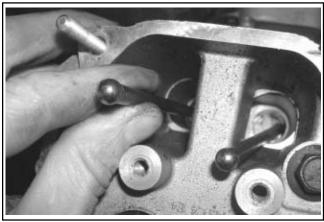
Figure 11-45. Install Push Rods in Their Original Position.
