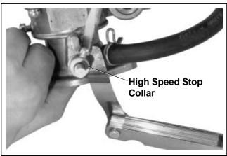
Figure 5A-12. Adjusting/Setting Stop Collar.
