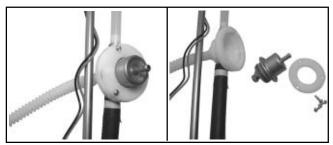
Figure 5B-31. Internal Regulator and Base/Holder.
