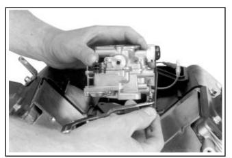
Figure 9-24. Removing Carburetor Assembly with Governor Lever Attached.
