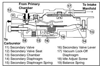
Figure 5A-22. Secondary Chamber.
