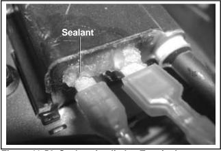
Figure 11-52. Sealant Applied to Terminals.
