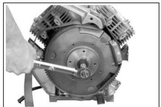
Figure 11-29. Installing and Torquing Flywheel Fastener.
