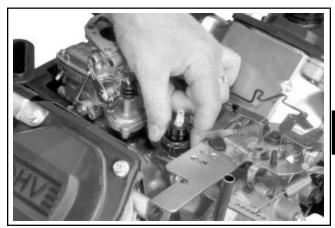
Figure 11-84. Installing Oil Sentry™ Switch.
