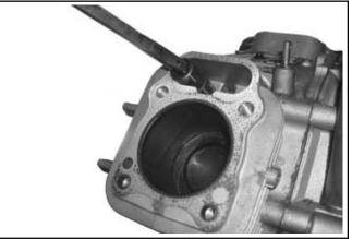
Figure 9-48. Removing Hydraulic Lifter.
