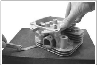
Figure 10-5. Checking Cylinder Head Flatness.
