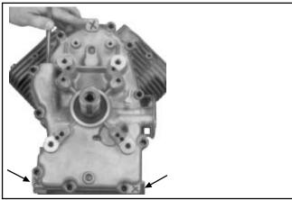
Figure 9-62. Location of Three Splitting Tabs.
