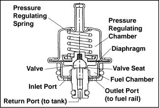
Figure 5B-29. Fuel Pressure Regulator Details.
