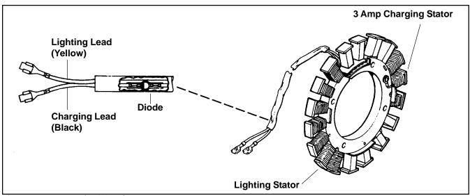
Figure 8-19. 3 amp/70 Watt Stator.
