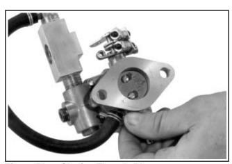
Figure 5A-9. Closing Throttle Plate.
