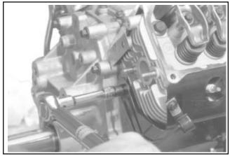
Figure 11-65. Tighten Baffle Mounting Screws.
