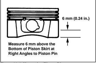
Figure 10-4. Measuring Piston Diameter.
