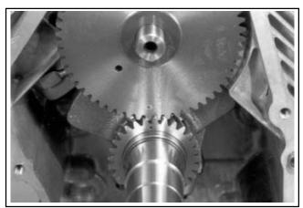
Figure 11-13. Aligning Crankshaft and Camshaft Timing Marks.
