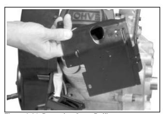
Figure 9-31. Removing Outer Baffles.
