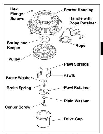
Figure 7-1. Retractable Starter - Exploded View.
