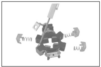
Figure 8-64. Removing Retaining Clips.
