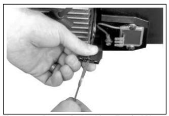
Figure 9-28. Remove B+ Lead from Terminal Plug.
