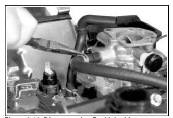
Figure 9-12. Disconnecting Fuel Inlet Line at Carburetor.
