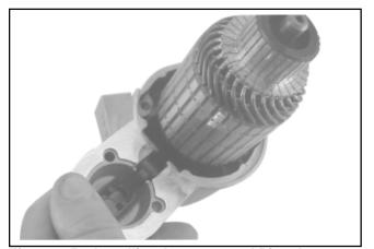
Figure 8-59. Installing Armature and Pivot Lever.
