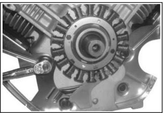
Figure 11-25. Installing Backing Plates and Stator Wire Bracket.
