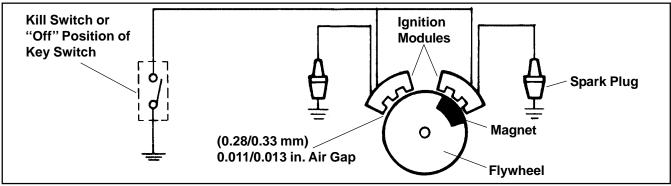
Figure 8-4. Capacitive Discharge (Fixed Timing) Ignition System.
