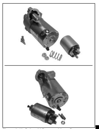
Figure 8-42. Solenoid Removed from Starter.
