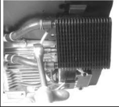
Figure 9-7. Removing Oil Cooler.
