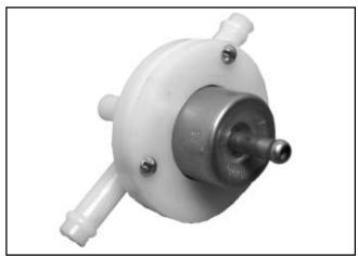
Figure 5B-28. Internal Fuel Pressure Regulator.
