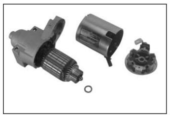
Figure 8-46. Starter Frame Removed.
