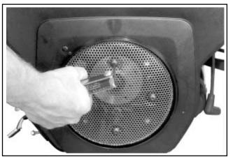
Figure 9-32. Removing Metal Grass Screen.
