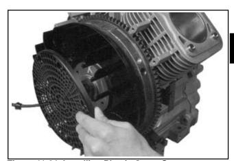
Figure 11-31. Installing Plastic Grass Screen.
