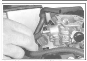
Figure 11-87. Connecting Fuel Inlet Line.
