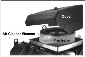
Figure 4-3. Removing Knob Style Cover.
