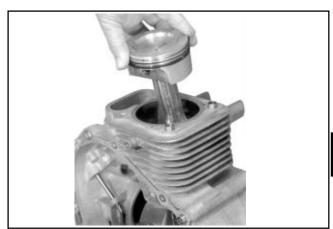
Figure 9-67. Removing Piston/Connecting Rod Assemblies.
