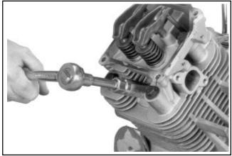
Figure 11-48. Installing Spark Plugs.
