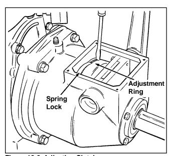
Figure 12-2. Adjusting Clutch.
