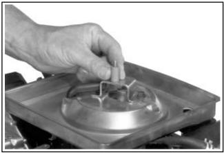
Figure 9-8. Removing Air Cleaner Base Retainer.
