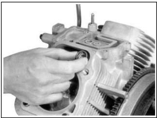
Figure 11-35. Installing Hydraulic Lifters.
