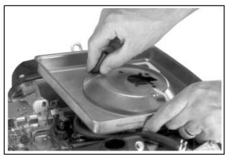
Figure 9-10. Removing Breather Tube from Base.
