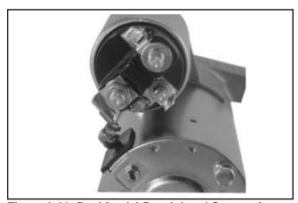
Figure 8-69. Positive (+) Brush Lead Connection.
