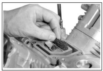
Figure 11-57. Installing New Breather Filter.
