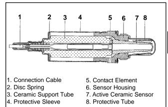
Figure 5B-12. Cutaway of Oxygen Sensor.
