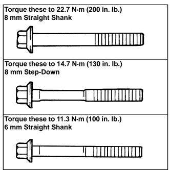
Figure 11-10. Connecting Rod Bolts.
