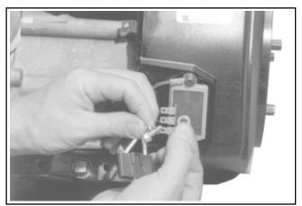
Figure 11-68. Connecting Ground Lead.
