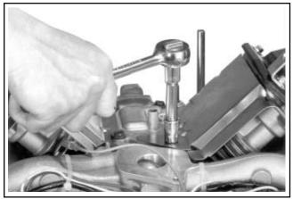
Figure 9-34. Removing Fasteners Holding Baffle and Breather Cover.
