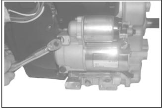
Figure 11-72. Installing Electric Starter Motor.
