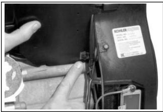
Figure 9-30. Note Location of Two Short Screws.
