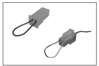
Figure 5B-9. Service Connector Plug, Plastic-Cased ECU Harness.
