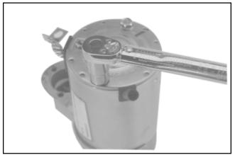
Figure 8-67. Torquing Thru Bolts.
