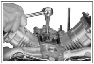
Figure 11-56. Installing Breather Reed Assembly.
