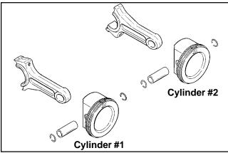
Figure 11-8. Piston, Connecting Rod and End Cap Detail.
