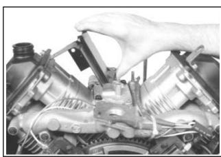
Figure 9-35. Removing Inner Baffles.
