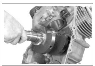
Figure 11-7. Installing Crankshaft.
