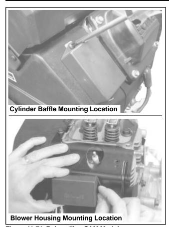
Figure 11-71. Reinstalling SAM Module.
