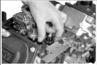
Figure 9-25. Removing Oil Sentry™ Switch from **Breather Cover.**
