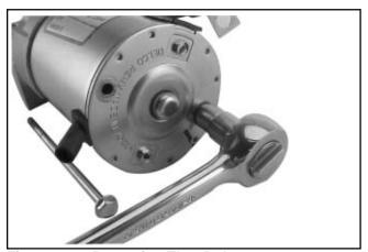
Figure 8-44. Removing Thru Bolts.
