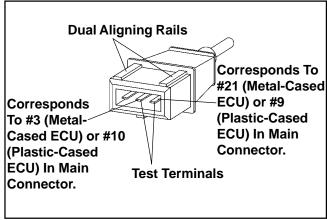
Figure 5B-5. Speed Sensor Connector.
