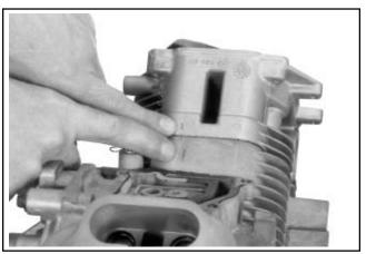
Figure 11-36. Match Numbers on Cylinder Barrel and Head.
