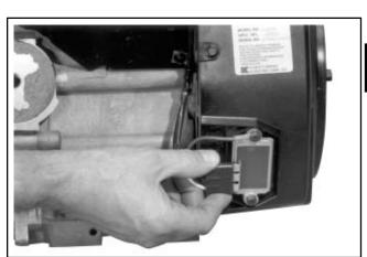
Figure 9-27. Disconnecting Plug from Rectifier-Regulator.
