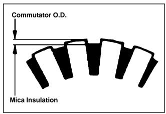
Figure 8-53. Commutator Mica Inspection.
