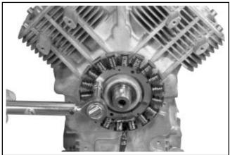
Figure 9-60. Removing Stator.
