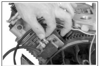
Figure 9-42. Position of SMART-SPARK<sub>™</sub> Ignition Module.
