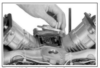
Figure 9-37. Removing Breather Cover.
