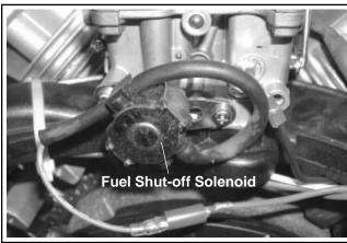
Figure 5-3. Fuel Shut-off Solenoid.
