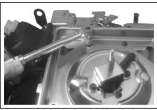
Figure 11-91. Tightening Rear Base/Bracket Screws (Some Models).
