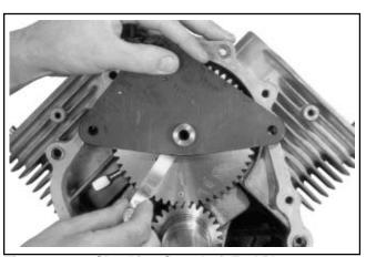
Figure 11-14. Checking Camshaft End Play.
