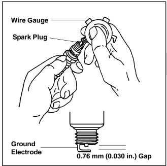
Figure 8-1. Servicing Spark Plug.
