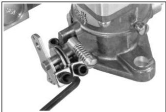
Figure 5A-14. Tightening Throttle Linkage Clamp
