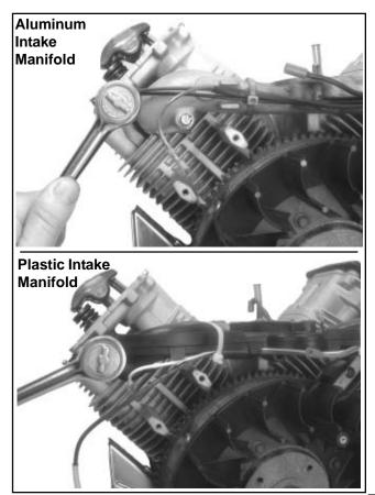
Figure 9-43. Removing Intake Manifold.
