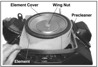
Figure 4-4. Air Cleaner Components.
