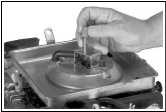
Figure 4-7. Removing Rubber Seal from Bracket.
