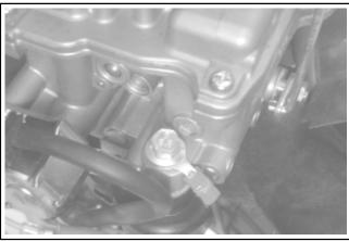
Figure 11-76. Ground Lead on Carburetor Mounting Screw.
