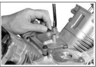
Figure 11-58. Installing Screws (Locations 3 and 4).
