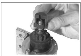
Figure 8-34. Assembling Larger Inner Half Around Spring Retainer.
