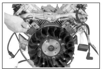
Figure 9-41. Disconnecting Leads from Ignition Modules.
