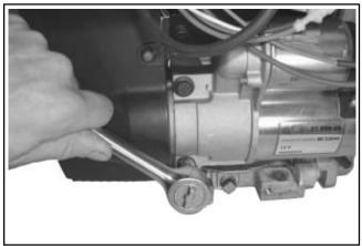
Figure 9-26. Removing Electric Starter Motor.
