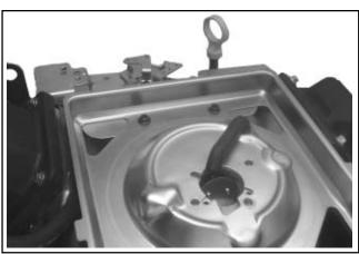
Figure 9-9. Rear Air Cleaner Bracket Screws.
