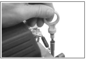
Figure 11-96. Reinstall the Dipstick in Tube.
