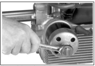
Figure 9-5. Removing Oil Filter.
