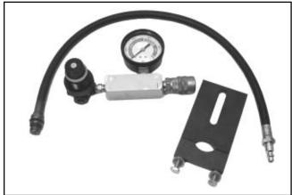
Figure 2-4. Cylinder Leakdown Tester.
