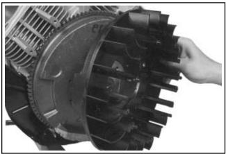
Figure 11-30. Installing Fan on Flywheel.
