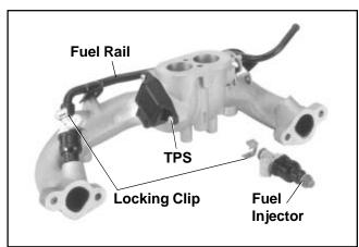
Figure 5B-33. Manifold Assembly.
