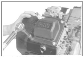
Figure 11-86. Tightening Valve Cover Screws.
