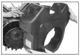
Figure 11-61. Installing Blower Housing.
