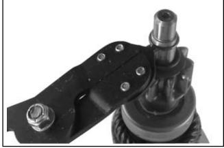
Figure 8-50. Removing Retaining Ring.
