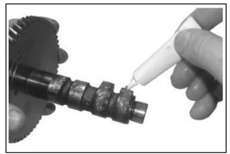
Figure 11-12. Apply Camshaft Lubricant to Cam Lobes.
