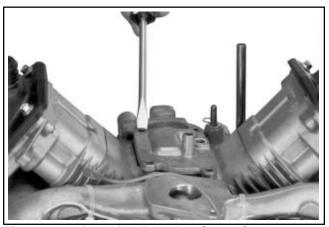
Figure 9-36. Breaking Breather Cover Seal.
