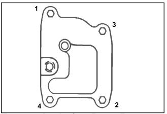
Figure 11-67. Breather Cover Fastener Torque Sequence.
