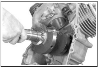
Figure 9-68. Removing Crankshaft.
