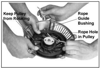
Figure 7-3. Installing Rope.
