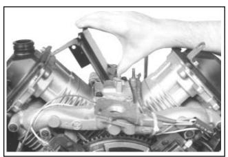
Figure 11-59. Installing Inner Baffles.
