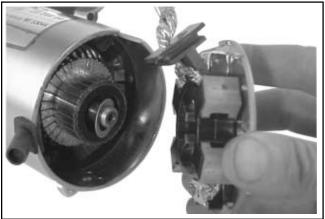
Figure 8-45. Removing Commutator End Plate Assembly.
