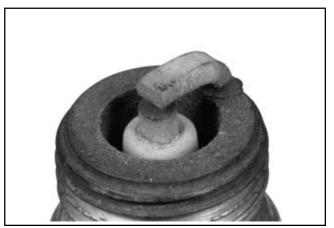
**Normal:** A plug taken from an engine operating under normal conditions will have light tan or gray colored deposits. If the center electrode is not worn, a plug in this condition could be set to the proper gap and reused.
