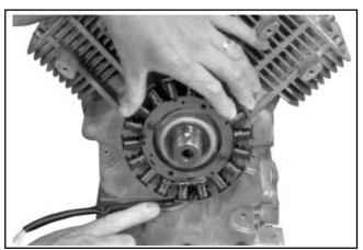
Figure 11-24. Route Stator Leads in Groove.
