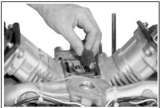
Figure 9-38. Removing Breather Filter.
