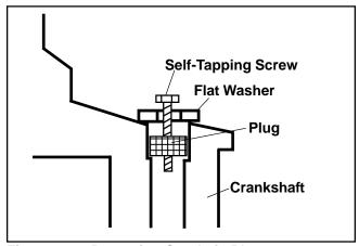
Figure 10-2. Removing Crankpin Plug.
