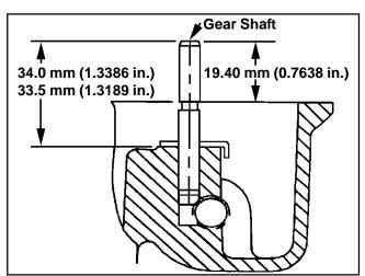
Figure 10-14. Governor Shaft Press Depth.
