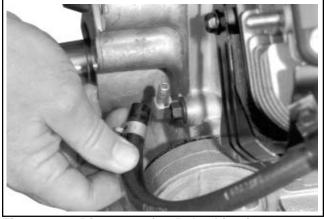
Figure 9-13. Disconnecting Pulse Line from Crankcase.
