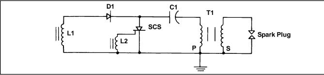
Figure 8-5. Capacitive Discharge Ignition Module Schematic.
