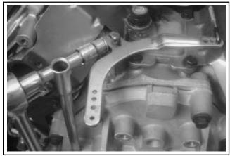
Figure 9-22. Removing Governor Lever.
