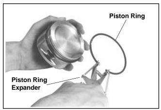
Figure 10-11. Installing Piston Rings.
