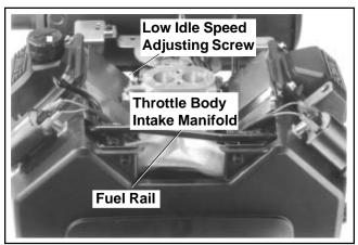
Figure 5B-35. Upper Intake Manifold.
