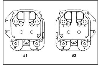
Figure 11-42. Cylinder Head Fastener Torque Sequence.
