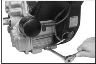
Figure 9-4. Removing Oil Drain Plug.
