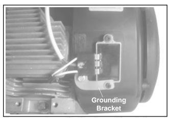
Figure 11-70. Grounding Bracket and Attached Connector.
