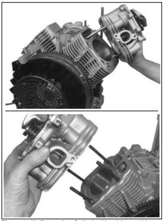
Figure 9-47. Removing Cylinder Head Assembly.
