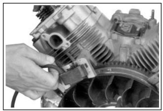
Figure 11-49. Installing Ignition Module.
