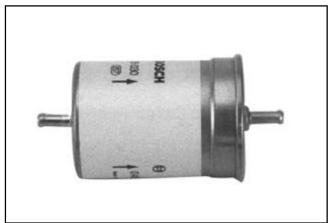
Figure 5B-32. In-Line Fuel Filter.
