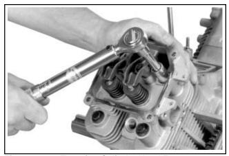
Figure 11-41. Torquing Cylinder Head Fasteners.
