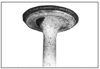
**Normal:** Even after long hours of operation a valve can be reconditioned and reused if the face and margin are in good shape. If a valve is worn to where the margin is less than 1/32" do not reuse it. The valve shown was in operation for almost 1000 hours under controlled test conditions.
