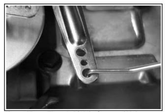
Figure 5B-40. Throttle Link in Center of Hole.
