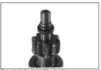
Figure 8-49. Retaining Ring Detail.
