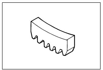
Figure 2-2. Flywheel Holding Tool.
