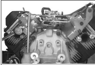
Figure 9-18. Removing Control Bracket.
