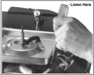
Figure 5B-19. Checking Injectors.
