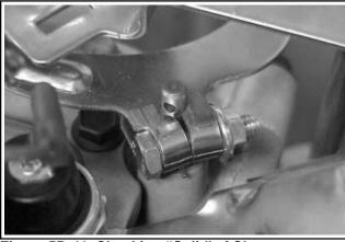
Figure 5B-41. Checking "Split" of Clamp.
