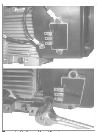
Figure 11-63. Ground Lead Details.
