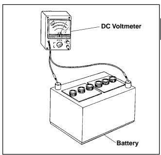
Figure 8-2. Battery Voltage Test.
