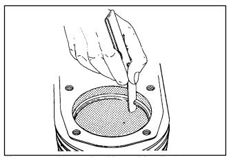
Figure 10-9. Measuring Piston Ring End Gap.
