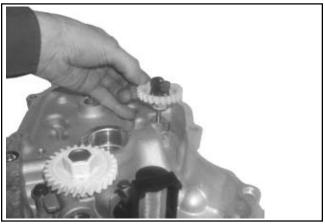
Figure 10-13. Removing Governor Gear.
