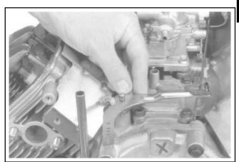
Figure 11-77. Install Governor Lever to Shaft.
