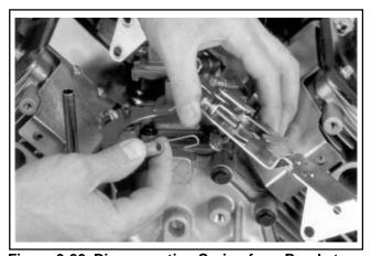
Figure 9-20. Disconnecting Spring from Bracket.
