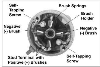
Figure 8-35. Style "A" Commutator End Cap with Brushes.
