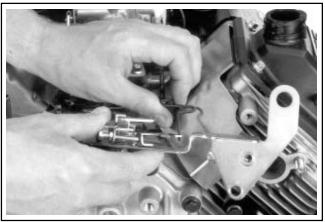
Figure 9-21. Disconnecting Choke Linkage from Actuator Lever.
