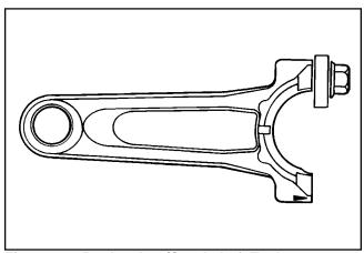
Figure 2-3. Rocker Arm/Crankshaft Tool.
