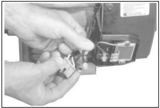
Figure 11-69. Installing B+ Lead into Plug.
