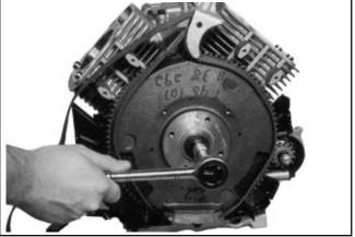
Figure 9-57. Removing Flywheel Fastener Using Strap Wrench.
