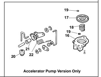
Figure 5-8. Carburetor - Exploded View.
