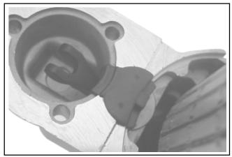
Figure 8-60. Installing Backup Washer and Grommet.
