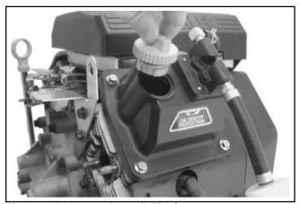
Figure 6-5. Removing Oil Fill Cap.
