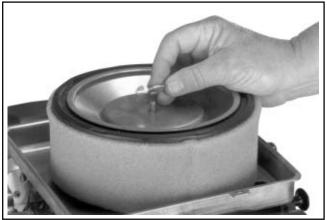
Figure 4-5. Removing Element Cover Wing Nut.
