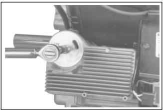
Figure 11-92. Torquing Oil Filter Nipple.
