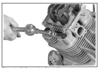
Figure 9-45. Removing Spark Plugs.
