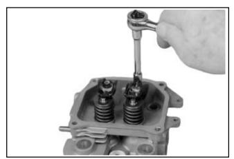
Figure 9-51. Removing Rocker Arms.
