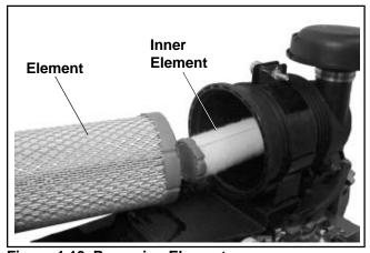
Figure 4-13. Removing Elements.
