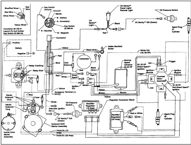
Figure 8-14. Wiring Diagram - 15/20/25 amp Regulated Battery Charging System.
