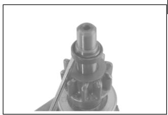
Figure 8-57. Installing Stop Collar and Retainer.
