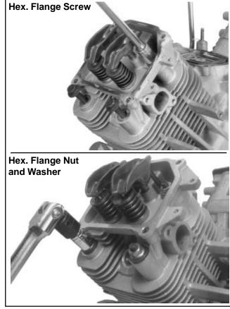
Figure 9-46. Removing Cylinder Head Fasteners.
