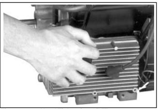
Figure 11-94. Hand Tightening Oil Filter.
