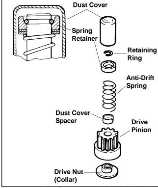
Figure 8-31. Drive Components, "Bonded" Inertia Drive Starter.
