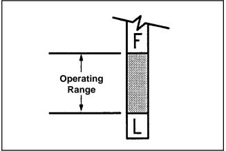
Figure 6-3. Oil Level Marks on Dipstick.
