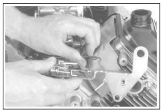
Figure 11-80. Connecting Choke Linkage.
