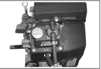
Figure 9-17. Mechanical Fuel Pump.
