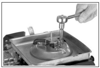
Figure 4-9. Bracket Retaining Screw.
