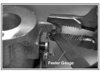
Figure 5B-39. Inserting Feeler Gauge (Engines Without Stop Screw).
