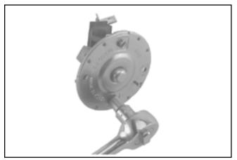
Figure 8-55. Removing Brush Holder.
