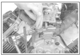
Figure 11-79. Holding and Tightening Governor Arm.
