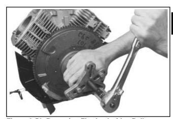
Figure 9-58. Removing Flywheel with a Puller.
