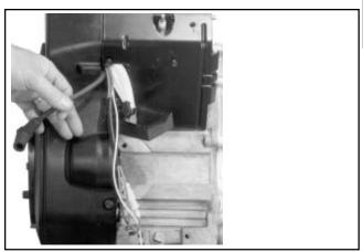
Figure 11-62. Routing Wiring Harness and Leads.
