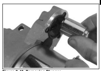
Figure 8-43. Removing Plunger.
