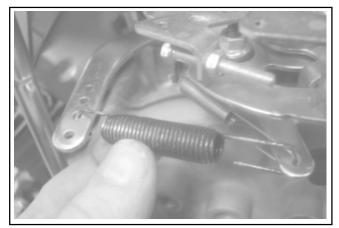
Figure 11-82. Connecting Spring to Governor Lever.
