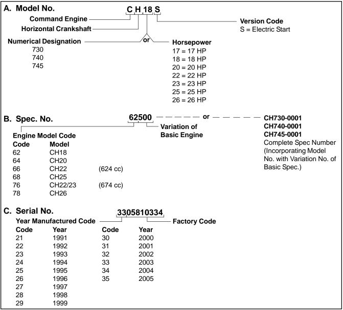
Figure 1-2. Explanation of Engine Identification Numbers.
