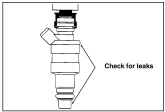
Figure 5B-21. Injector Inspection Points.
