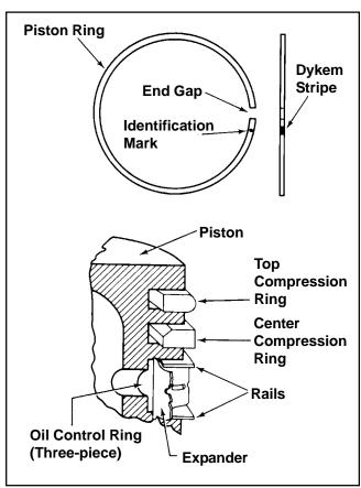
Figure 10-12. Piston Ring Installation.
