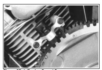
Figure 5B-4. Engine Speed Sensor.
