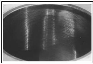
Figure 10-3. Cylinder Bore Crosshatch after Honing.
