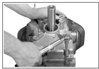
Figure 11-22. Torquing Closure Plate Fasteners.
