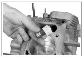
Figure 9-49. Mark Position of Hydraulic Lifters.
