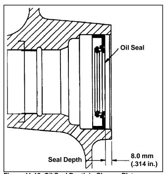
Figure 11-18. Oil Seal Depth in Closure Plate.
