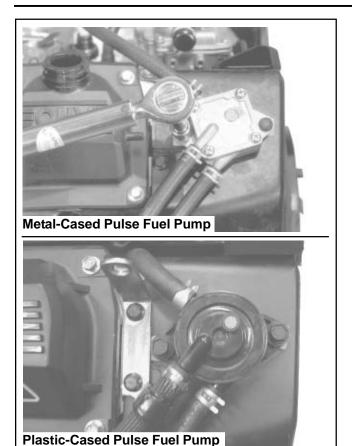
Figure 11-74. Reinstalled Fuel Pump.
