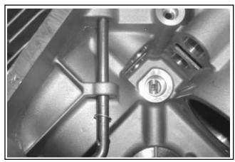
Figure 11-5. Installing 8 mm Governor Cross Shaft.
