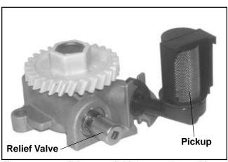
Figure 10-16. Oil Pump, Oil Pickup, and One-Piece Relief Valve (Later Style).
