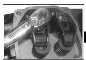
Figure 11-46. Torquing Rocker Arm Screws.
