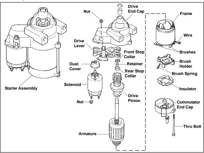
Figure 8-39. Nippondenso Solenoid Shift Starter.
