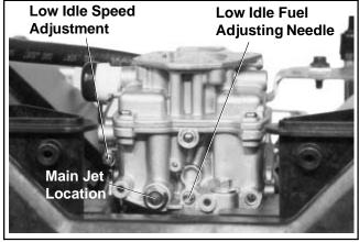
Figure 5-4. Pre-Compliance Carburetor with Low Idle Adjustment.
