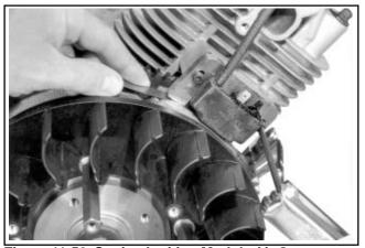
Figure 11-50. Setting Ignition Module Air Gap.
