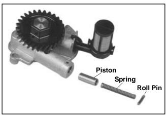
Figure 10-17. Oil Pressure Relief Valve Piston and Spring.
