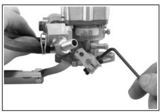
Figure 5A-10. Tightening Idle Speed Clamp Mounting Screw.
