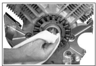
Figure 11-26. Clean and Dry Taper of Crankshaft.
