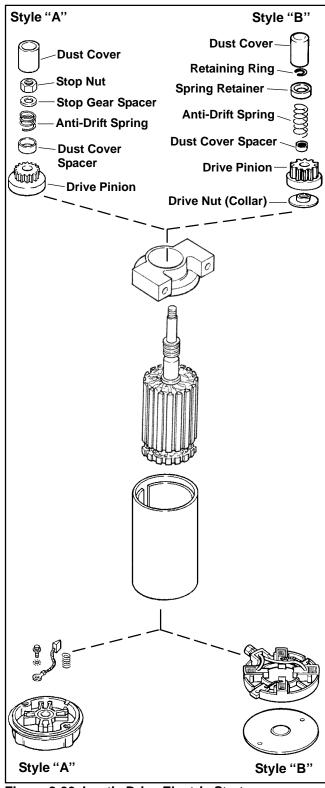
Figure 8-30. Inertia Drive Electric Starter.
