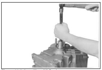
Figure 11-2. Installing Oil Seal.
