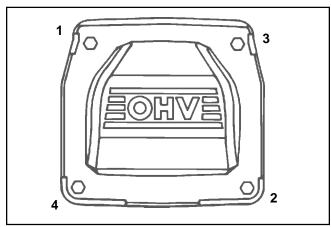
Figure 11-85. Valve Cover Fastener Torque Sequence.
