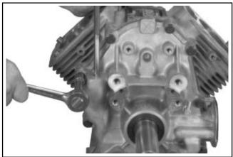
Figure 9-61. Removing the Ten Closure Plate Fasteners.
