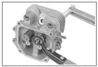
Figure 9-52. Removing Valves with Valve Spring Compressor.
