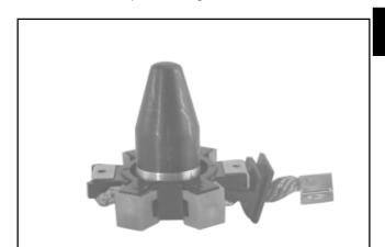
Figure 8-65. Brush Installation Tool with Extension.
