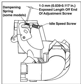
Figure 5B-36. Idle Speed Screw Details.
