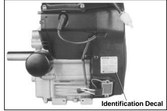
Figure 1-1. Engine Identification Decal Location.
