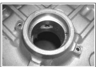
Figure 11-1. Seal Bore of Crankcase.
