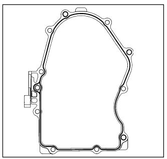
Figure 11-19. Closure Plate Sealant Pattern.
