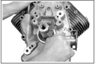
Figure 11-20. Using Spanner Wrench to Turn Crankshaft.
