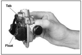
Figure 5-7. Carburetor Float Adjustment.
