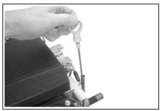
Figure 9-2. Removing Dipstick from Tube.
