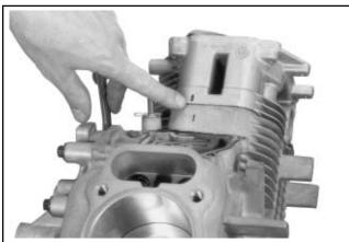
Figure 9-50. Match Marks on Cylinder Barrel and Heads.
