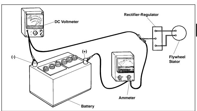
Figure 8-29. Connections for Testing Charging System.
