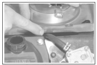
Figure 11-89. Fuel Inlet Line Detail.
