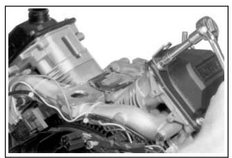
Figure 9-40. Removing Valve Covers.
