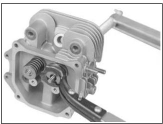
Figure 11-39. Installing Valves with Valve Spring Compressor.
