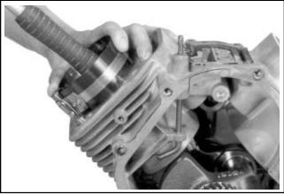
Figure 11-9. Installing Piston Assembly Using Ring Compressor Tool.
