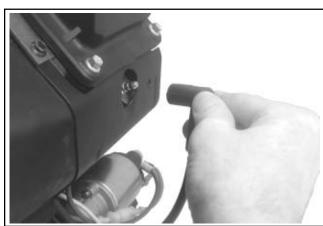
Figure 9-1. Disconnect Both Spark Plug Leads.
