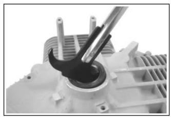
Figure 9-72. Removing Oil Seal.
