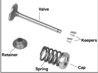
Figure 11-38. Valve Components.
