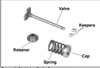
Figure 9-53. Valve Train Components.
