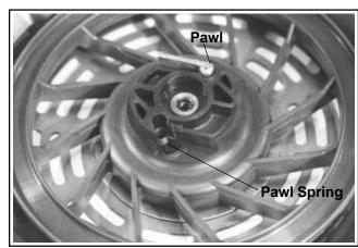
Figure 7-9. Installing Pawls and Pawl Springs.
