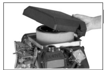
Figure 4-2. Removing Latch Style Cover.
