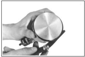
Figure 10-10. Measuring Piston Ring Side Clearance.
