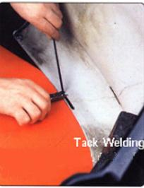
A Tack welding nozzle 28 (push fitted onto the standard nozzle of the **BAK RION**) is used at the temperature specified for the material (see table). The weld is best completed in one continuous run from end to end, drawing the welding nozzle tip along the base of each 'V' groove.
