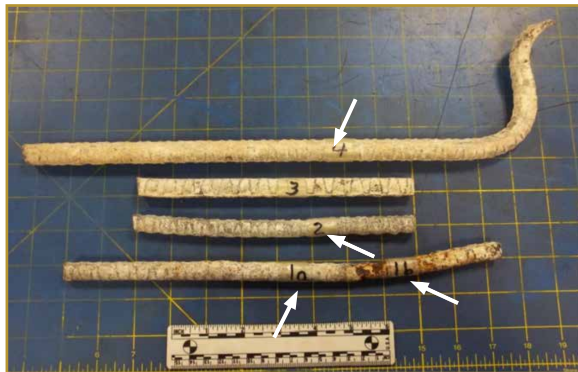
Figure 1. As-received galvanized rebar sections showing the locations of the samples removed for metallographic examination and optical coating thickness readings.
