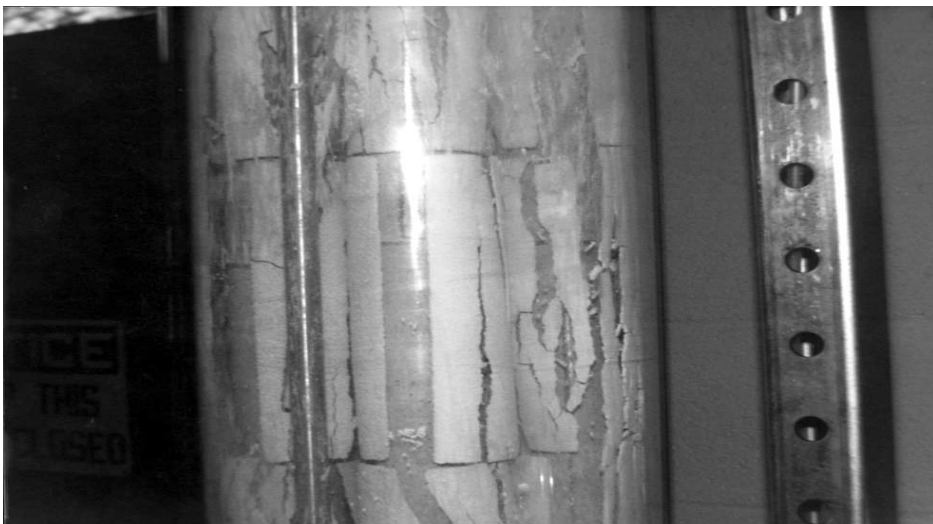
Figure 4. Photograph of cake release during pulse blowback.
