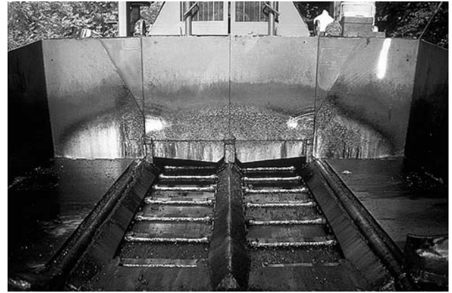
FIGURE 15-5 Slat conveyors at bottom of paver hopper.
