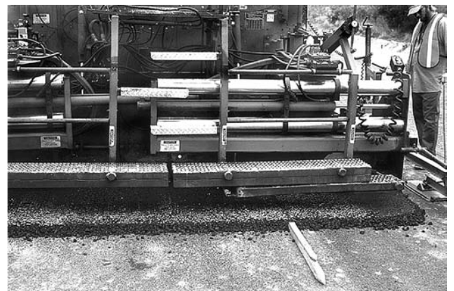
FIGURE 15-21 Hydraulically extendable screed.
