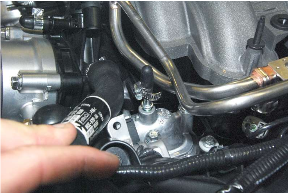
Push and hose clamp the small coolant barb behind the 3/4" coolant tubes.
