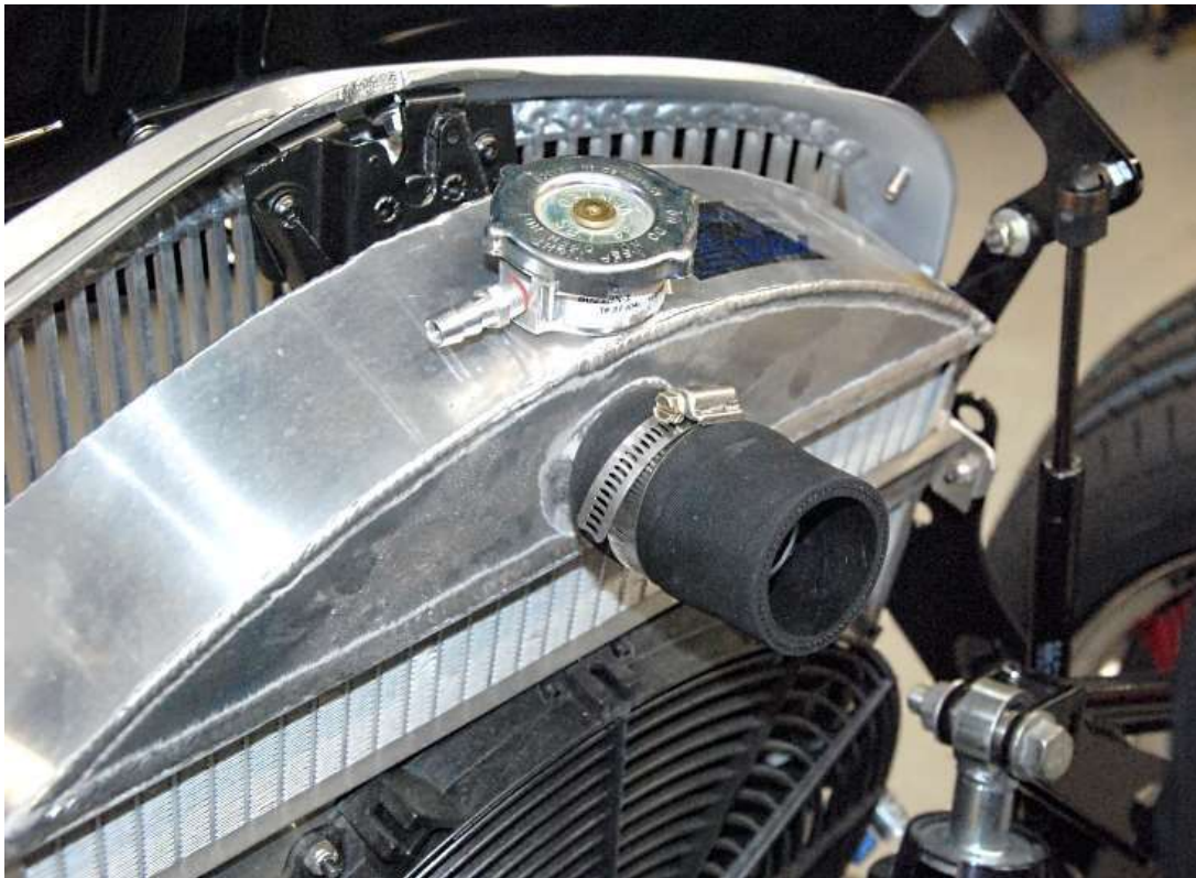
Attach another hose adapter to the radiator.
