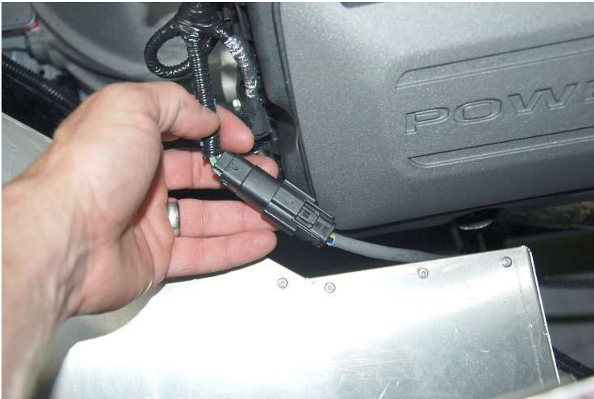
Attach the right O 2 sensor to the connector at the back of the head.
