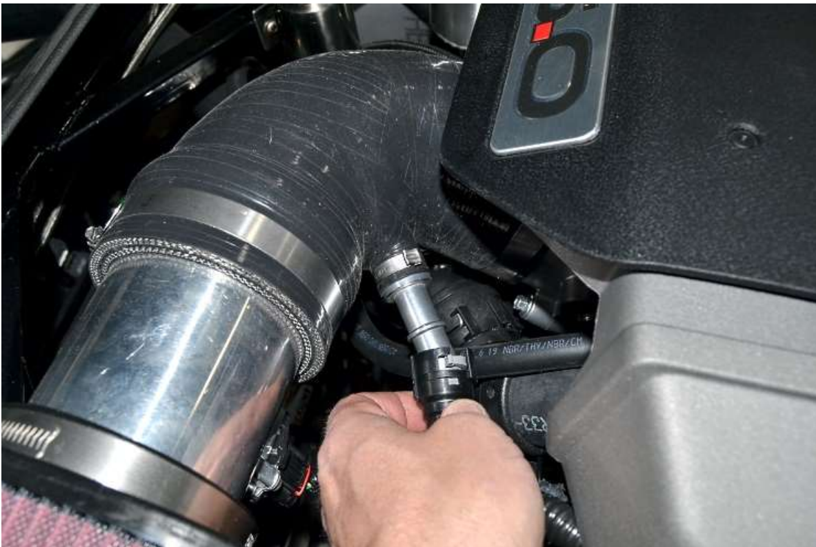
Attach the other end of hose to the intake hose.
