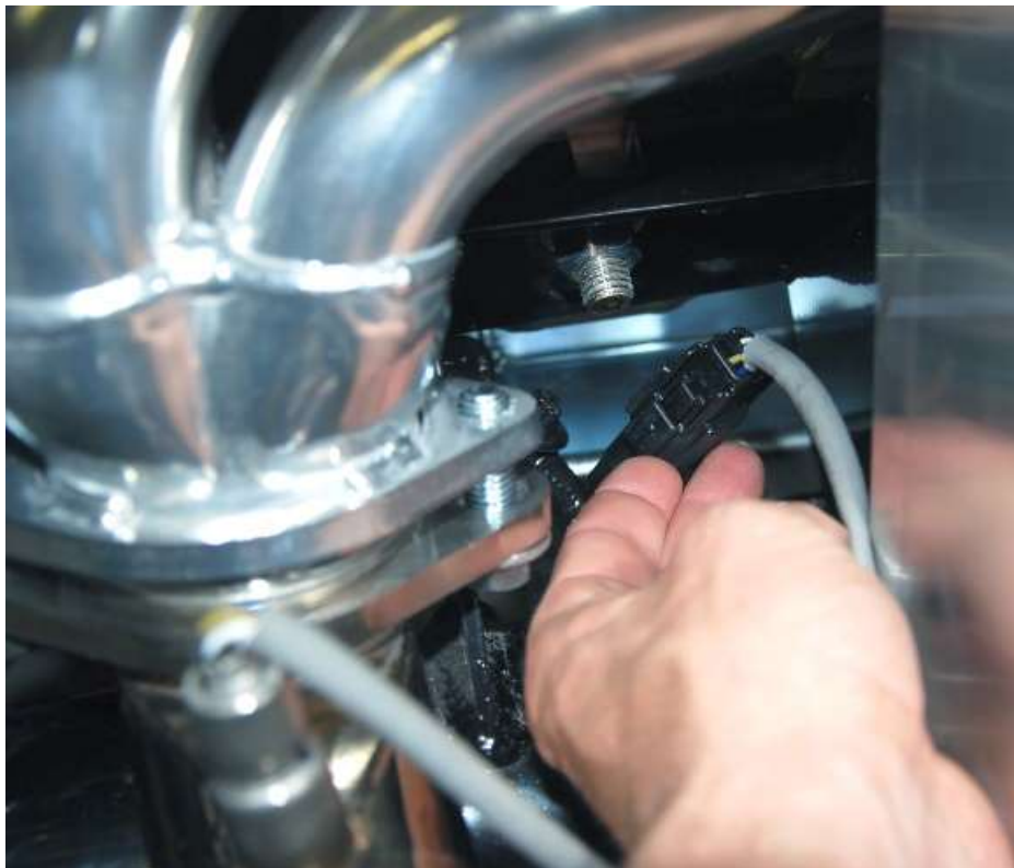
Connect the left O 2 sensor to the connector down near the engine mount
