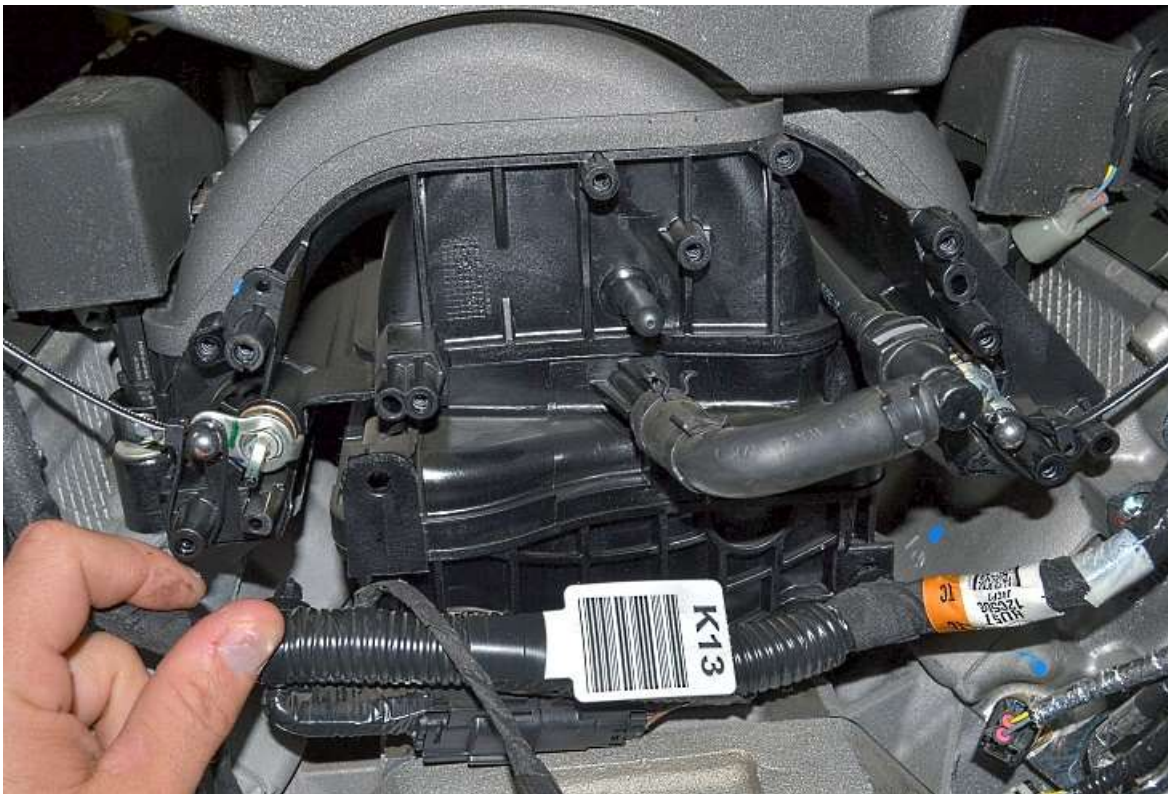
When standing in behind of the engine, the left side CMCV shaft needs to be rotated counterclockwise and locked in position.
