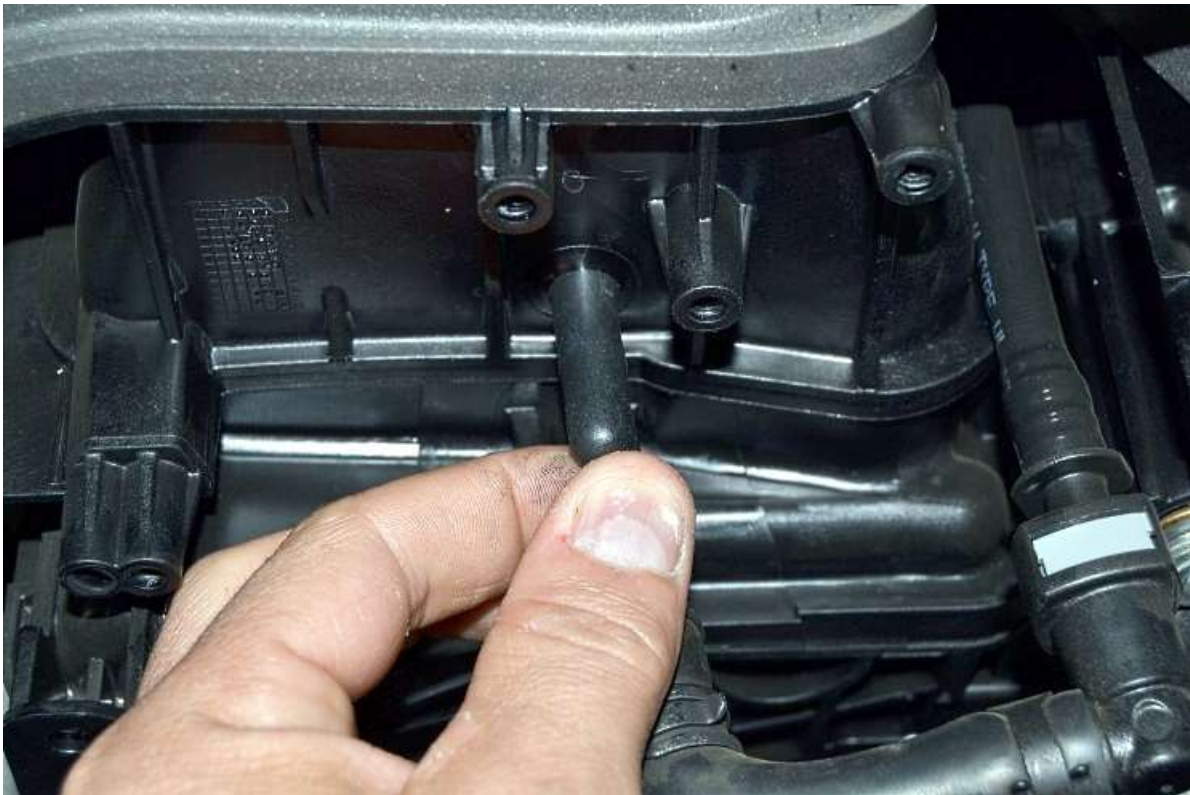
Cap the vacuum nipple above the just shortened.
