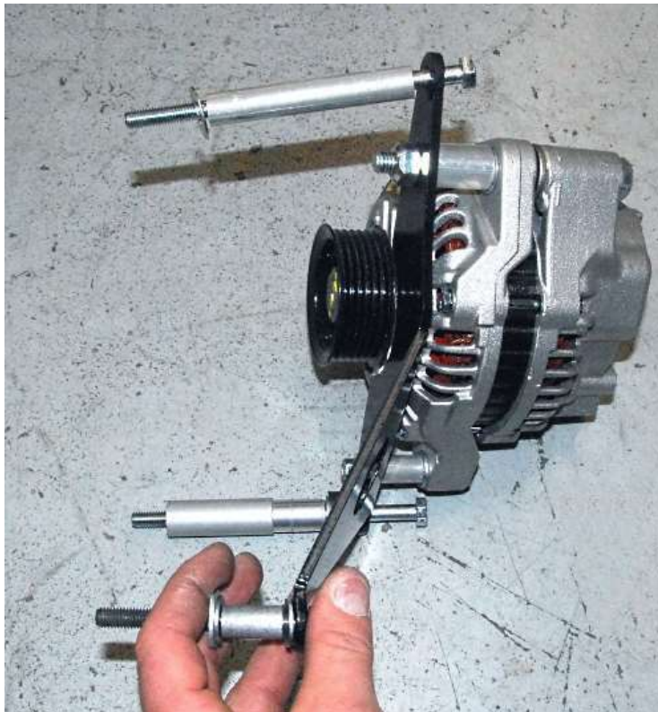
Run the bracket mounting bolts through the bracket and put the spacers on the bolts.
