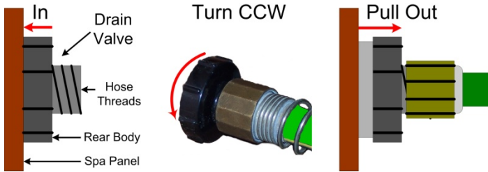
Figure 26 - Drain Operation
