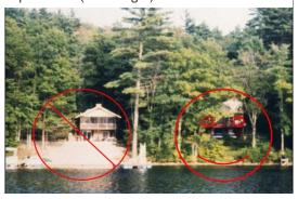
The waterfront house on the right has a view and direct water access, but incorporates vegetative buffers to slow and filter runoff before it enters the lake, unlike the house on the left.
