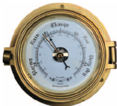
Figure 2.3 A mechanical gauge used to measure atmospheric pressure. In general, mechanical gauges work via an air-filled tube that changes shape with changing pressure. Levers and/or gears move in response to the tube, and a pointing needle and scale or an electronic display is calibrated to show the corresponding atmospheric pressure. From Cracolice, M. S., & Peters, E. I. (2011). Introductory Chemistry: An Active Learning Approach . Belmont, CA: Brooks/Cole Cengage Learning.
