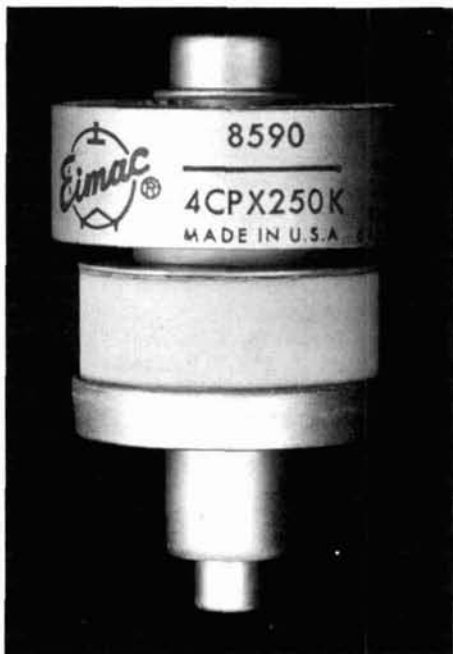
Tube designed for large phased-array radar system. Two of these tubes were used in the 1000-watt 432-MHz amplifier used by WAGLET with a 150-foot dish for moonbounce contacts in 1965.
