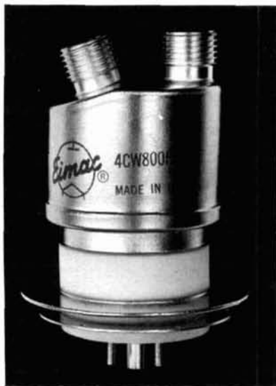
Distributed-amplifier tube discussed in text. By choosing the number of control-grid leads, the designer can control lead inductance. The tube in the right-hand photo has a screen by-pass capacitor installed. Center pin is one of the heater pins; the square tab on the capacitor is the other heater connection and the cathode. The threaded pins are control-grid leads.
