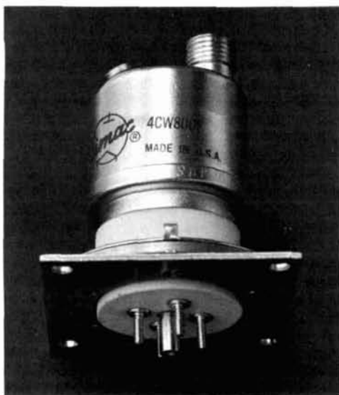
Distributed-amplifier tube discussed in text. By choosing the number of control-grid leads, the designer can control lead inductance. The tube in the right-hand photo has a screen by-pass capacitor installed. Center pin is one of the heater pins; the square tab on the capacitor is the other heater connection and the cathode. The threaded pins are control-grid leads.
