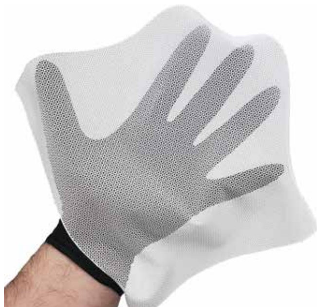
Figure 10. A sheet of Dimension Inx’s 3D-printed Hyperelastic Bone, which is flexible despite being 90% ceramic.
