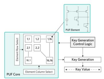
Figure 3. Block diagram of Maxim Integrated's ChipDNA PUF architecture.
