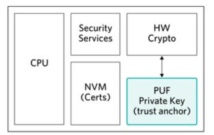
Figure 6. PUF as trust anchor private key.
