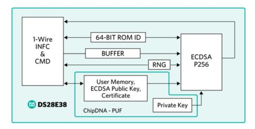
Figure 7. Block diagram of Maxim's ChipDNA PUF-based ECDSA authenticator.
