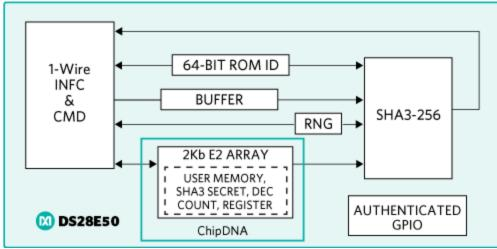
Figure 8. Block diagram of Maxim's ChipDNA PUF-based SHA3 authenticator.
