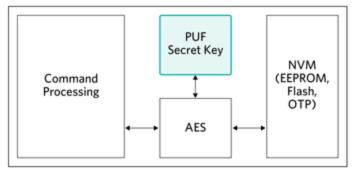
Figure 4. Encrypting IC NVM with the PUF secret key.
