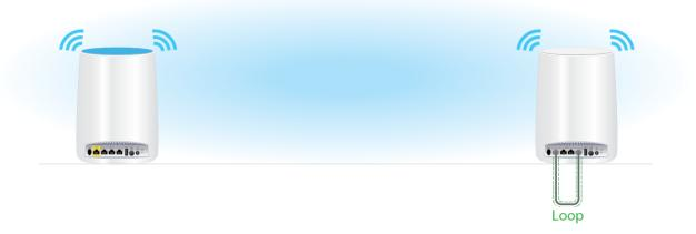
**Problem:** Both ends of an Ethernet cable are plugged into the same Orbi Satellite.
