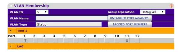
4. In the VLAN Membership section, confirm that default VLAN 1 now displays that ports 1-10 and port 12 are untagged (U), as shown in this image:
