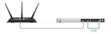
**Problem**: Both ends of an Ethernet cable are plugged into the same network switch.
