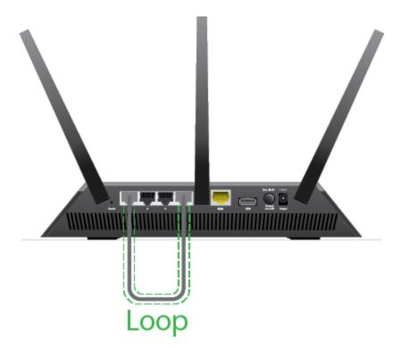
**Problem**: Both ends of an Ethernet cable are plugged into the same router.
