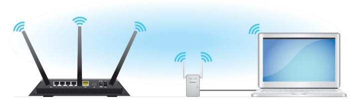
**Problem**: A wireless device is connected to a wireless extender using an Ethernet cable, but the device's WiFi is not turned off. The wireless device could be an IP camera, a computer, a smart home hub, or any other device that supports both wired and wireless connections.
