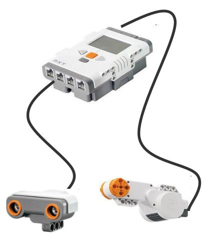
Do This: Connect the LEGO brick to the ultrasonic sensor and a motor, as shown to the left.
