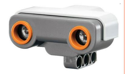
The air pressure vibrations makes the diaphragm move in that microphone, and this diaphragm motion is sensed and converted into an electrical signal (like the sound sensors you have studied). The time lag between the sent and received sound is used by the brick to estimate the distance to the object. As mentioned before, this is how bats also estimate distance.
