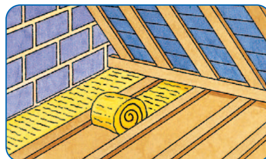
Insulating the loft with glass fibre 20 cm thick can save half of the thermal energy lost through the ceiling.
