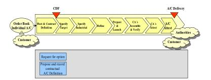
Figure 4: Specification and production of an individual aircraft
