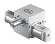
The Bimba Pneu-Turn® position feedback rotary actuator (PTF) provides continuous shaft position sensing. Standard features include shaft ball bearings and the elimination of mid-rotational backlash. Use the Bimba PTF in conjunction with Bimba's Pneumatic Control System (PCS) to achieve rotary shaft positioning accuracy within  $\pm 0.5^{\circ}$ .
