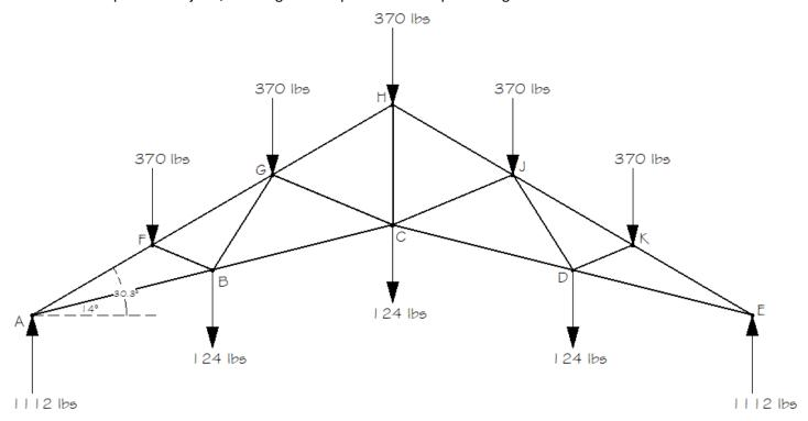
The wall at A exerts a force of 1112 lbs vertically, and a force of 0 lbs horizontally at A, which members AF and AB must work together to counter. Let's assume members AF and AB are pulling away from A in tension.
