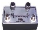
A PreAmp to raise very small signals to a level can be captured by a PC sound card.
