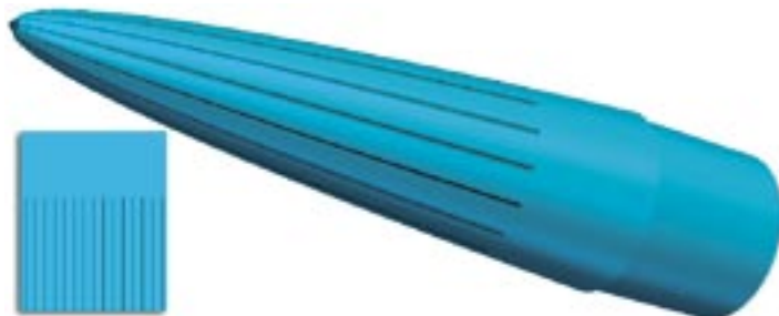
Figure 14: RockSim will conform the rectangular pattern to the shape of the nose cone.
