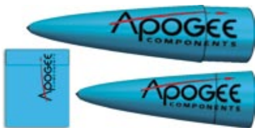
Figure 12: The wrap can span the shoulder of the nose cone if you allow it. The same artwork was applied to both noses. Note the shoulder line on the artwork.
