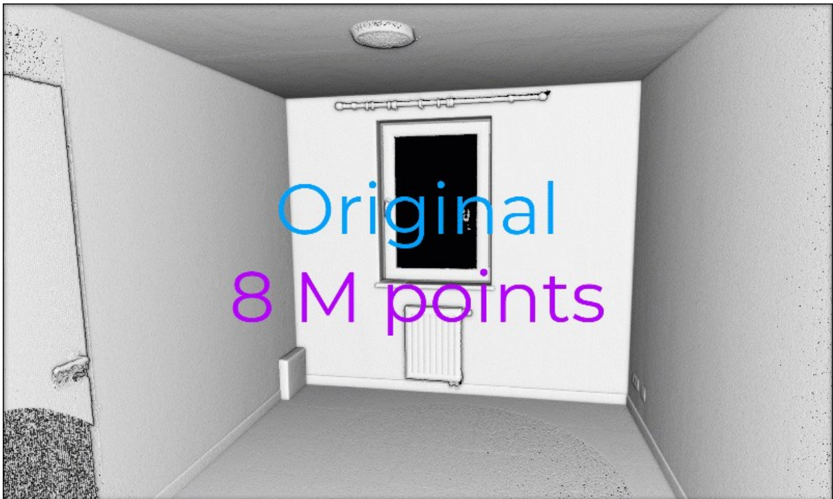
The point cloud is sampled using a voxel grid, with different voxel sizes. For each voxel, one representative point is retained. © Florent Poux
