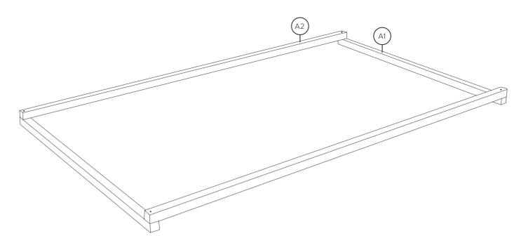
5. Attach the wooden blocks with nails in the same way as the pictured example.
