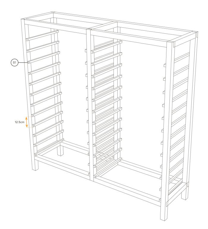
4. Attach the wooden blocks with nails in the same way as the pictured example.
