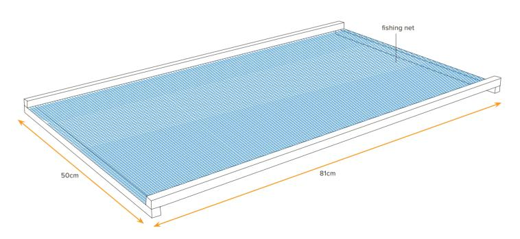
6. Attach the fishing net to the shelf frame with thumb tacks in the same way as the pictured example.
