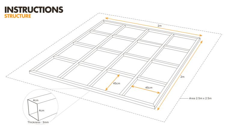
1. Prepare an area of 2.5mx2.5m. Ensure that the area is flat by using a split level and is free from rocks and grass.
