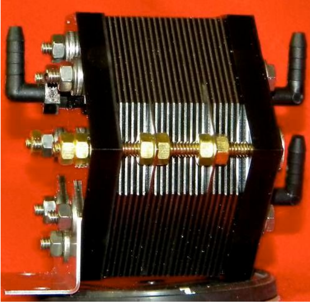
Larger HHO generating cell, be sure your barb fittings will fit a 3/8" hose, if not you will need to replace the hose barb.
