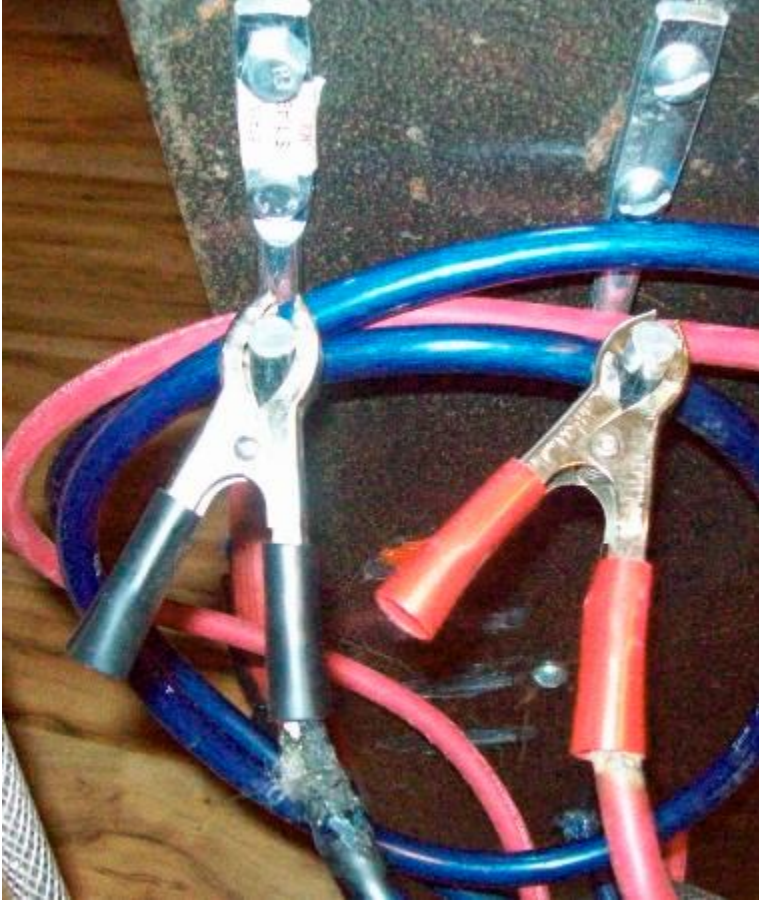
Close up of the power connectors for my HHO heater/cooker
