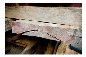
Checking happens when a board dries too quickly or unevenly. The cracks move along the board. So it's best to avoid these boards. If you are cutting your own lumber from a tree, checking can often be prevented by using a good quality wood end grain sealer (like I mentioned above)...the red stuff painted on the ends of boards in many of the above & below photos. Lumber should also be stacked with "stickers" or spacers of even thickness, with weights on top.
