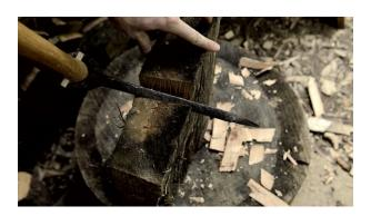
The most stable boards are "riven" or "rived" directly from a log by <u>you</u>, exploiting the weakness of the grain (like splitting firewood). Riven boards are a subset of quartersawn because they are also split along the radial plane of the log, producing grain lines that are square to the board face and straight down the board.
