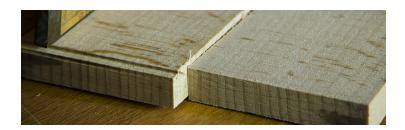
Quartersawn wood is very stable, and less susceptible to movement. The 60-90 degree verticle grain qualifies a board as "quartersawn" within the lumber industry. See how the end grain is running nearly up-and-down? That is called "vertical grain". Quartersawing also produces fairly straight face grain and usually very beautiful ray flecks (for example, see the flecks on the beech wood above).
