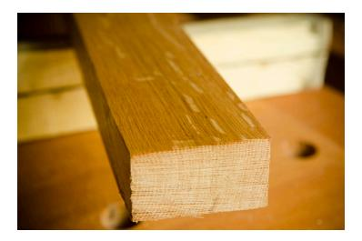
So why do you not hear about this type of lumber very often? Because wood mills and lumber yards don't have it. Their boards are cut with large powerful saws. Riven boards require muscle power and hand tools like a large crosscut saw (or chain saw), wedges, mallets, a froe, an adze, a hewing hatchet & handplanes.
