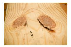
Knots can cause problems for hand tool woodworkers, especially when passing your handplane over the top. And knots like to fall out over time. Yes, you can mix epoxy and sawdust to solidify the knot, but most of the time I avoid them all together. But you may like the look of them in a rustic piece of furniture. Just be aware.
