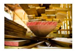
When green (wet) boards aren't properly stacked they will cup or twist. Cupping is when the board turns into a cup shape (see above). Twisting is when board ends twist different ways. It takes a lot of work to plane out the twisting or cupping. I don't always turn down free wood that is twisted or cupped, but I won't buy it.
