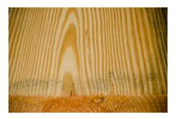
Notice how the above  $2\times12$  construction-grade flat sawn board actually has some very stable quartersawn wood on both sides of the wide board? Here's what it looks like after I cut it off with a rip saw and use handplanes to square it up:
