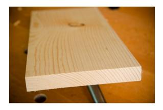
The riftsawn section of a board is similar to quartersawn cuts, but its endgrain is between 30-60 degrees to the face. Riftsawn boards have a characteristically straight face grain pattern. These boards are also pretty stable and can be utilized if your furniture project calls for extremely straight face grain, like modern or Japanese-style projects.
