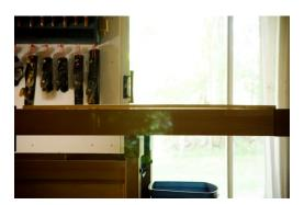
Bowed boards are like a bow that you shoot arrows with (see above). To me, this defect is a bit harder to correct for than twisting or cupping. So I avoid these boards...unless they're free (like the above lacewood board was).
