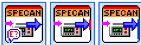
Fig. 5-8: Fast Write icons: with Error Checking / with OPC? synchronisation / with *WAI synchronisation.
