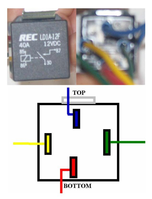
Yellow will go to the Start Relay yellow wire, Blue goes to ballast resistor with the Dark Green/Red wire, Green goes to ground, and Red goes to the red battery wire on the Start Relay.
