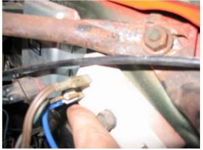
Yellow Wire – This wire hooks up to the yellow Trans Neutral Switch wire on the Starter Relay.
