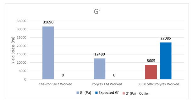
*Figure 6* shows the expected G' values and the actual G' values for the 50:50 mixture of Chevron SRI Grease 2 to Mobil Polyrex EM and the reference greases.
