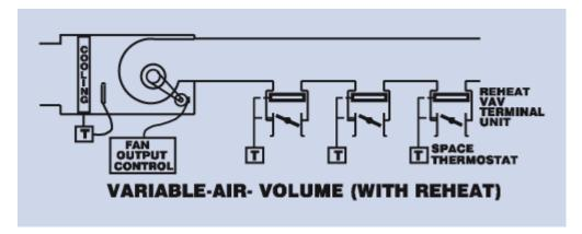
Figure 1 VAV System Schematic<sup>2</sup>
