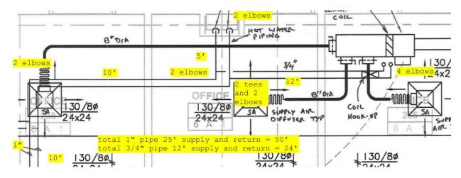
Figure 2 Taylor Engineering Mechanical Drawing Excerpt<sup>9</sup>
